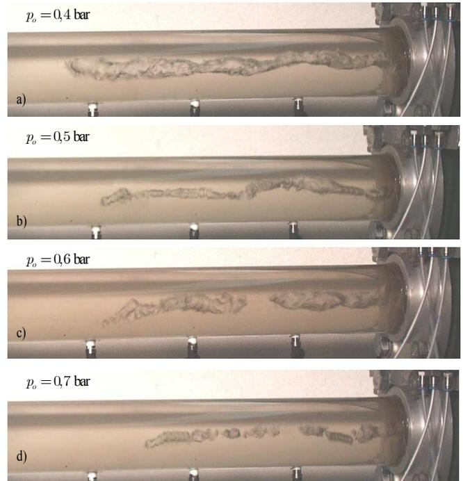
Fig. 8: Cavitation swirl tearing and reducing its diameter with pressure in the reservoir
