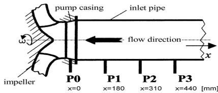
Fig. 6: Measuring places at the pump entrance
