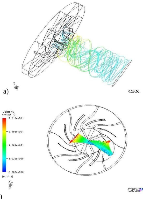
b) Fig. 1: Streamlines (a) and vector plot (b) of flow swirl at the fan entrance eye
