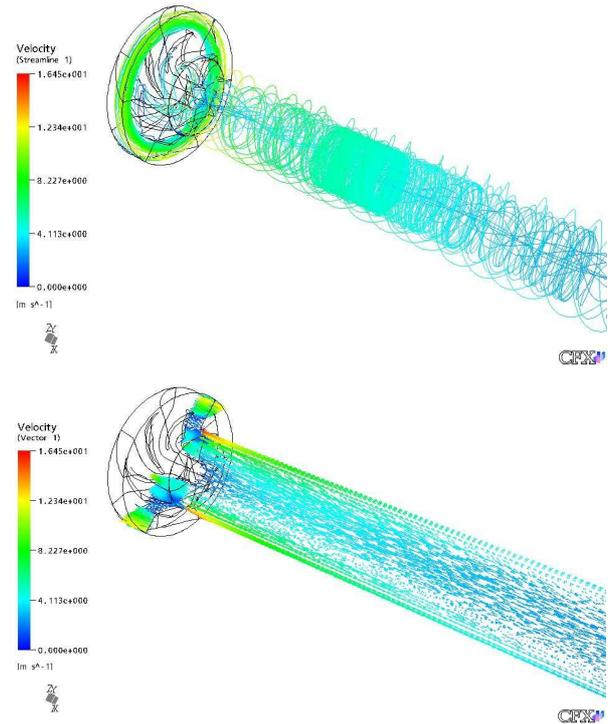
Fig. 4: Cavitation swirl flow pattern - streamlines and vector plot.
