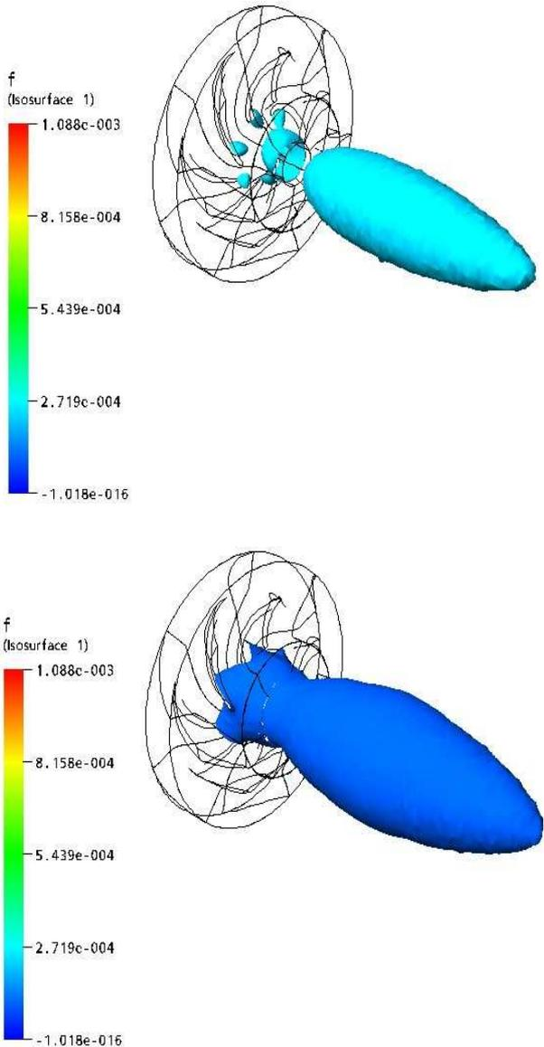
Fig. 3: Cavitation swirl vapour fraction (isosurface plot)
