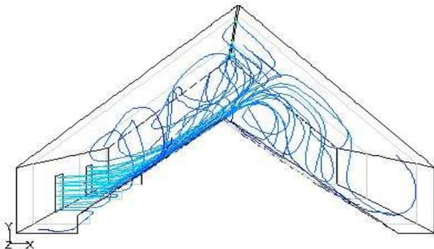
Fig.3 Coal depot ventilation by the door opening - flow paths
