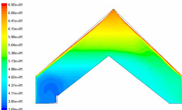
Fig.4 Temperature distribution inside the coal depot in the scale between 36°C and 69°C - results of 2-D model
