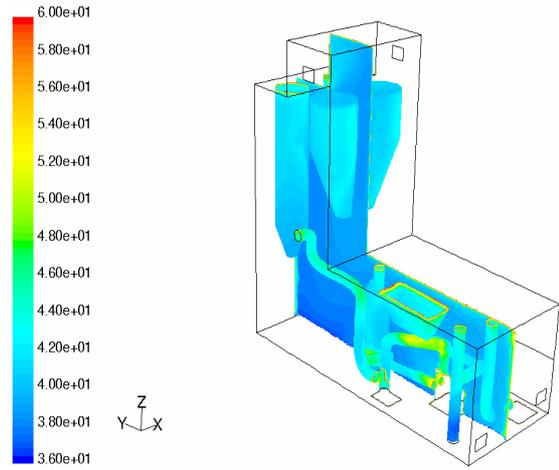
Fig.9 Temperature distribution inside the coal mill in the scale between 36°C and 60°C at  $x = 7$  m - results of 3-D model
