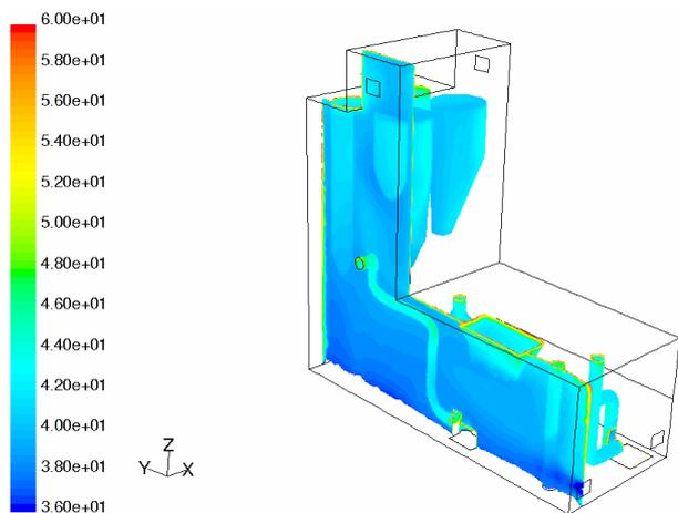
Fig.8 Temperature distribution inside the coal mill in the scale between 36°C and 60°C at  $x = 2$  m - results of 3-D model
