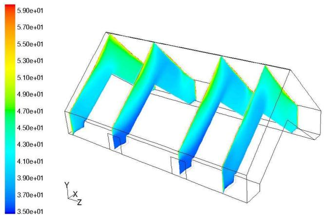
Fig.6 Temperature distribution inside the coal depot in the scale between 35°C and 59°C - results of 3-D model
