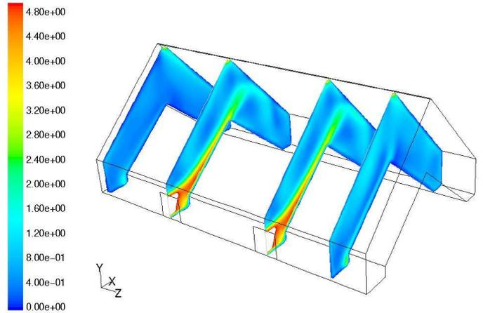
Fig.5 Velocity distribution inside the coal depot in the scale between 0 and 4,8 m/s - results of 3-D model
