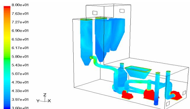
Fig.2 Surface temperatures of the equipment within the coal mill in the scale between 36°C and 80°C
