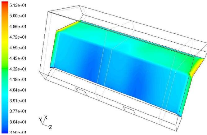
Fig.7 Temperature distribution in the boundary layer close to the coal pile - scale between 35°C and 55°C - results of 3-D model
