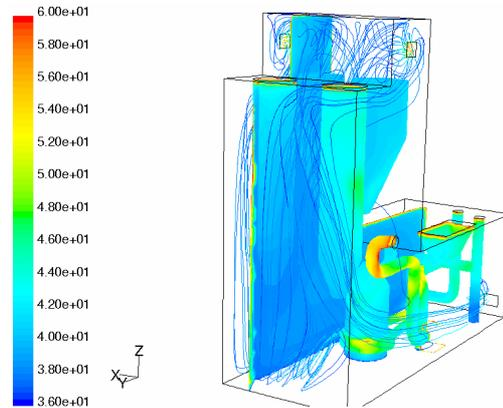
Fig.10 Air flow path - lines and temperature distribution inside the coal mill in the scale between 36°C and 60°C at  $x = 12$  m - results of 3-D model
