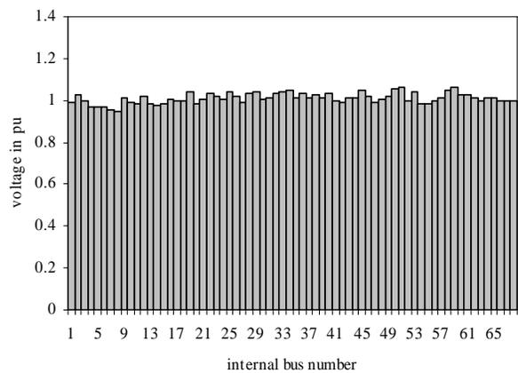
**Fig. 3. Bus voltage magnitude profile of the stressed system after placing 145 MVar SVC at bus 40.**
