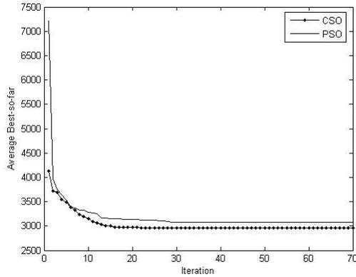
**Fig. 4. Convergence characteristics of CSO and PSO on the average best-so- far in finding the solution, 145 MVar SVC at bus 40.**
