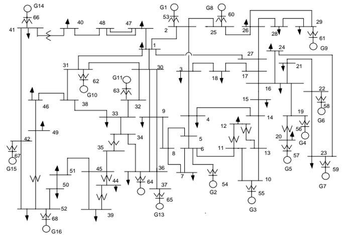
**Fig. 1. Single line diagram of a 5-area study system.**
