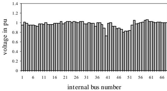
**Fig. 2. Bus voltage magnitude profile when system is heavily stressed.**
