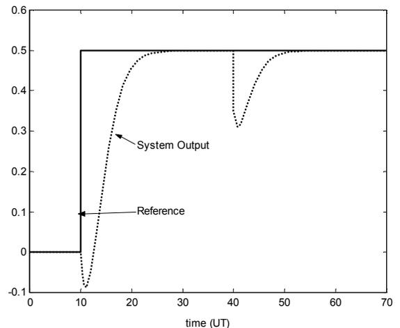
Figure 5. Process response to set point and disturbances changes
