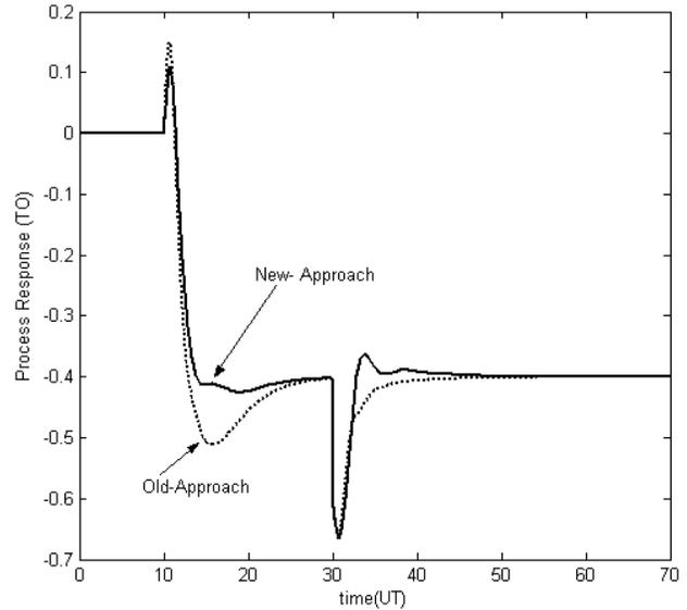
Figure 7. Process responses for set point and disturbance changes, using both controllers.
