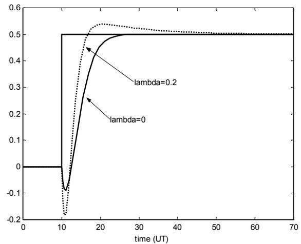
Figure 4. Closed loop response for  $\lambda=0.2$  and  $\lambda=0$
