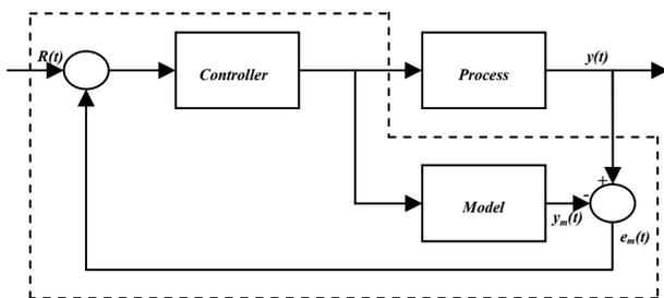
Figure 1. Internal Model Structure
