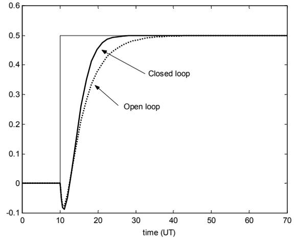
Figure 3. Open and Closed loop responses
