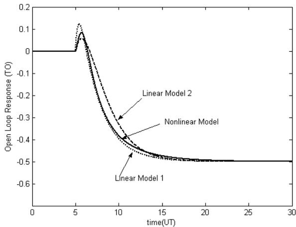
Figure 6. Open loop responses of nonlinear and linear models.
