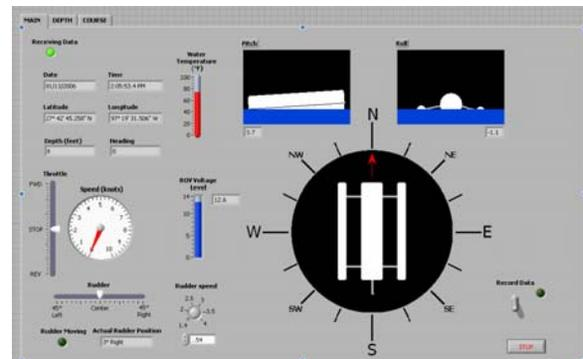
Fig. 4 GUI while ROV is running
