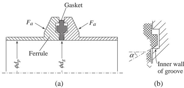
Figure 1: The SUSDETOP<sup>®</sup> metal gasket. (a) A schematic view of a pipe joint assembled with two ferrules ( $F_a$ : assembly force). (b) An enlarged view of the seal area.
