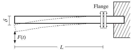
Figure 2: A cantilevered structure of pipe.
