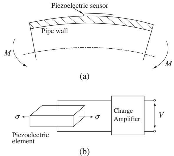
Figure 4: (a) A piezoelectric thin film sensor adhered to a pipe to measure stress of the pipe wall. (b) Transversal effect of a piezoelectric element.
