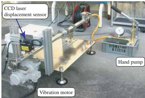
Figure 3: An example of the proposed vibration testing rig.
