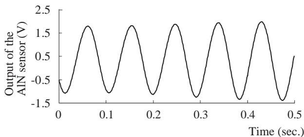
Figure 7: Examples of signals of AlN piezoelectric sensor.
