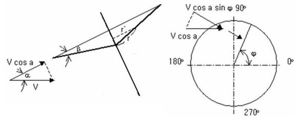
Figure 3: Velocity vectors in blades of the Chinese top.
