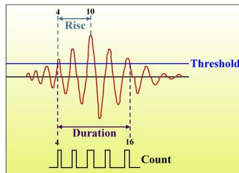
Fig. 4. Explanatory Drawing of Feature Value
