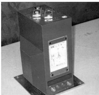
Fig. 5 Experimental tailor-made cast-resin transformer
