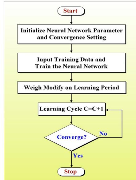
Fig. 10. Training Process Chart of Artificial Neural Network
