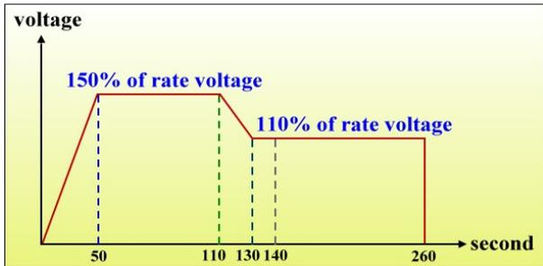
Fig. 9. Explanatory Drawing of Voltage Test Procedure
