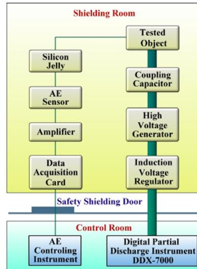
Fig. 1. Diagram of PD Measurement Structure for AE
