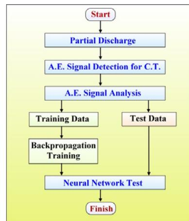
Fig. 2. Flowchart of the proposed PD Defect Classification Process
