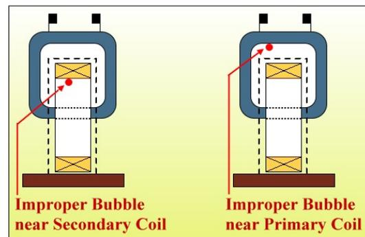
Fig. 8. Improper Bubble within Insulating Material on Low and High-Voltage Side
