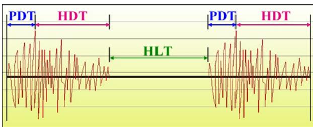
Fig. 3. Drawing of Acoustic Emission Wave Definition
