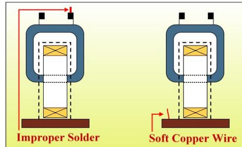
Fig. 7. Improper Solder on High-Voltage Side and Improper Soft Wire on Grounding Panel
