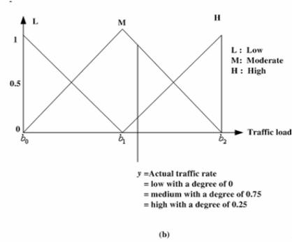
Figure 3: Example for the fuzzification of the system parameter (a) the number of available channel and (b) traffic loads.
