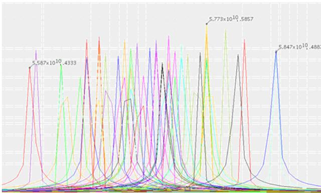
Fig.5 Monte Carlo simulation at 57 GHz
