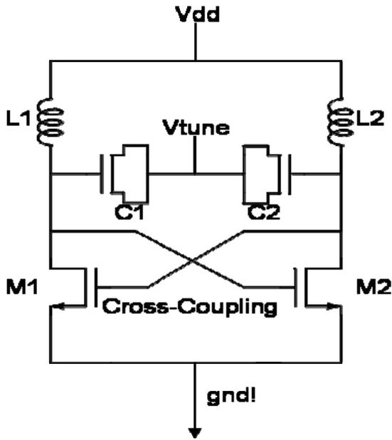
Fig.1 VCO core structure
