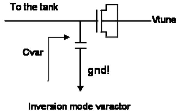
Fig.3 NMOS transistor with source and drain connected together to act as an inversion mode capacitance.
