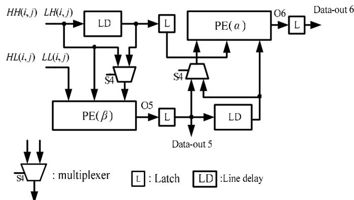
Fig. 10. The architecture of Inverse vertical filter (IVF)
