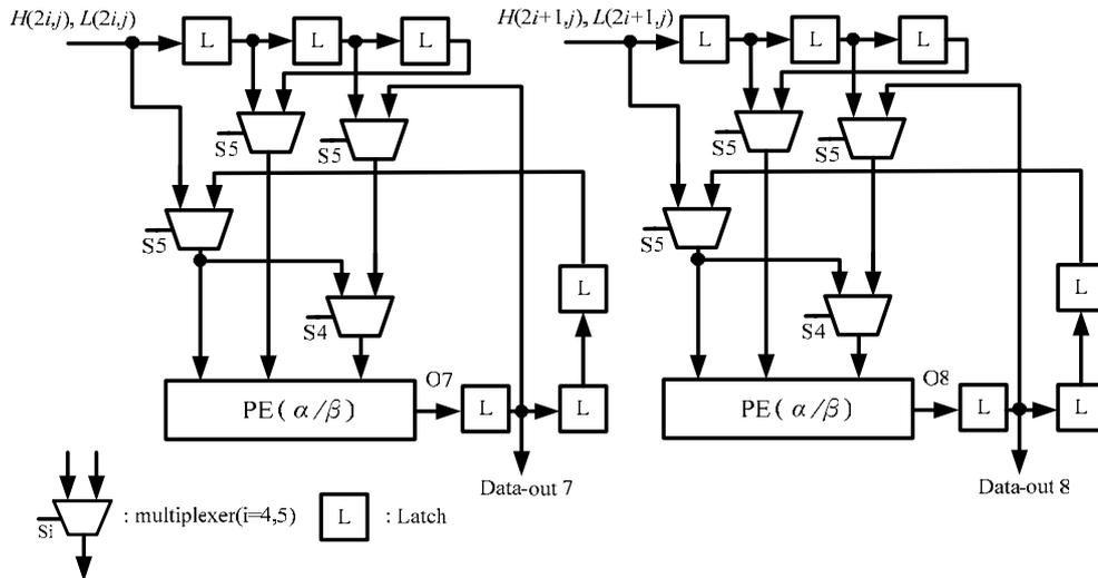
Fig.11. The architecture of inverse horizontal filter (IHF)
