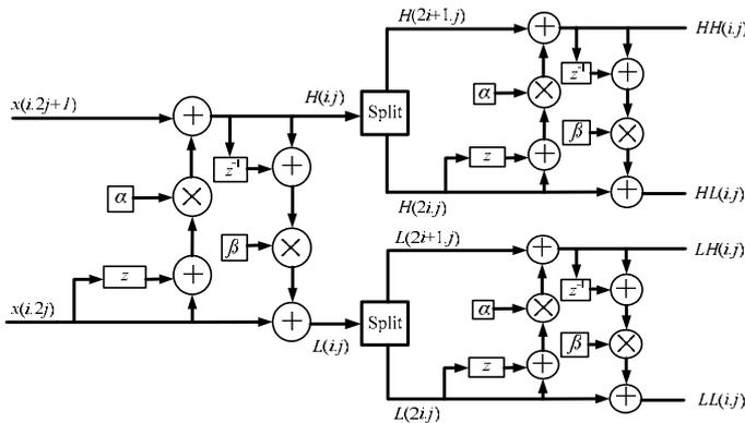
Fig.3. 5/3 2-D lifting-based DWT
