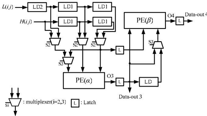
Fig.6. The architecture of vertical filter (VF)
