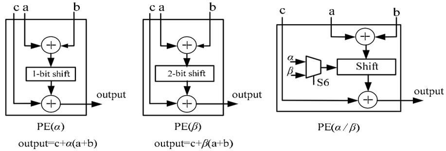
Fig. 12. The architectures of  $PE(\alpha)$ ,  $PE(\beta)$  and  $PE(\alpha/\beta)$
