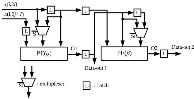
Fig.5. The architecture of horizontal filter (HF)
