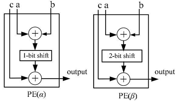
Fig. 8. The architectures of  $PE(\alpha)$  and  $PE(\beta)$
