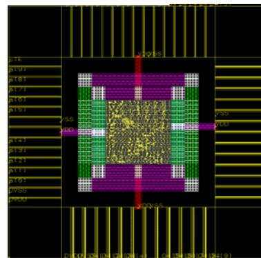
Fig.14. Layout view of the proposed 2-D IDWT core processor
