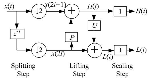
Fig.1. The architecture of DWT based on lifting scheme
