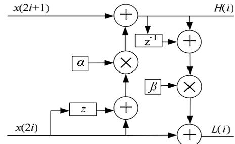
Fig.2. 5/3 1-D lifting-based DWT
