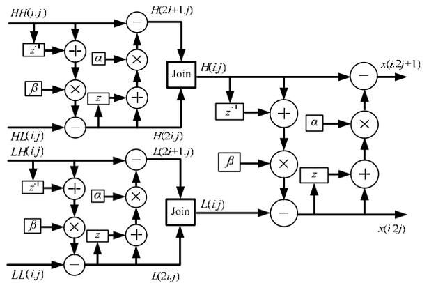
Fig.9. 5/3 2-D lifting-based IDWT
