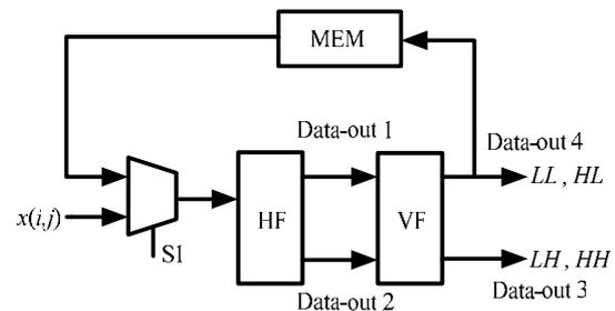
Fig.4. The proposed system architecture of 5/3 2-D lifting-based DWT
