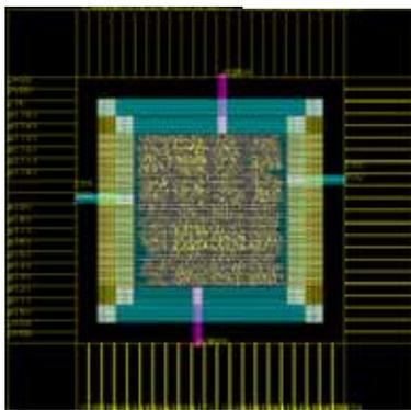
Fig.13. The Layout view of the proposed 2-D DWT core processor
