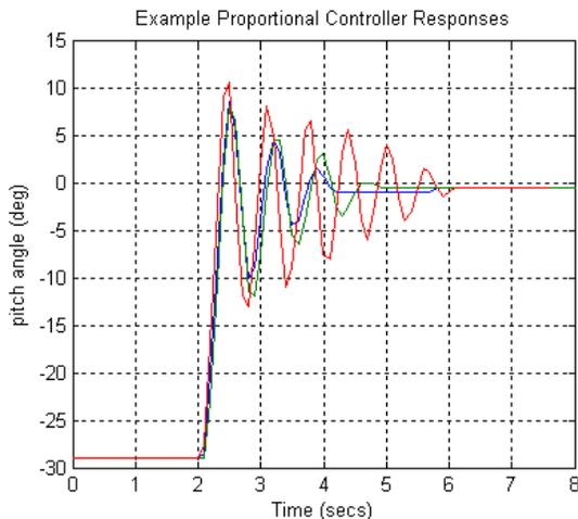
Figure 3 Experimental Transient Responses-Proportional controller only
