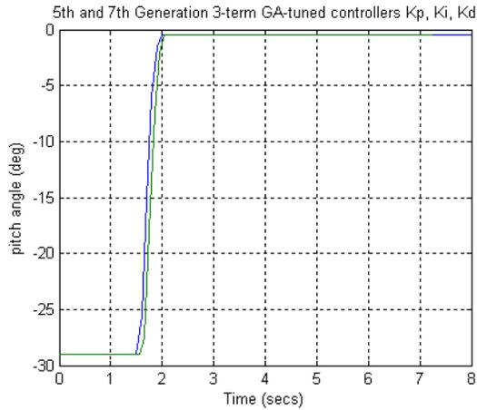
Figure 6 Experimental Transient Responses-GA tuning of PID, 5<sup>th</sup> and 7<sup>th</sup> generation results
