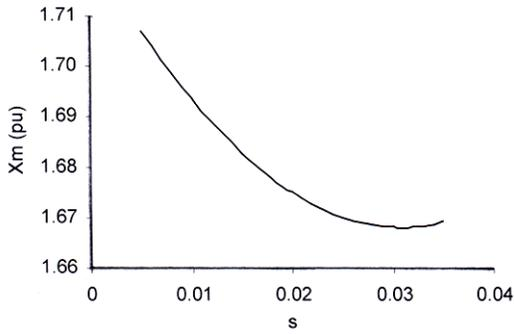
Fig.8 Variation of magnetizing reactance with slip
