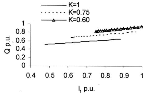
Fig. 11 Variation of reactive power with stator current, terminal voltage =  $1.1 V_1$ , magnetizing reactance= $K X_{mu}$
