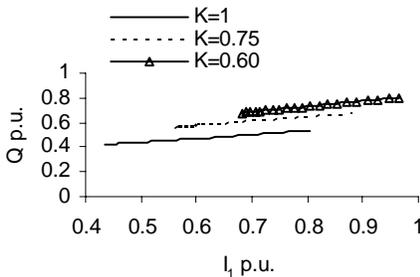
Fig. 10 Variation of reactive power with stator current, terminal voltage =  $V_1$ , magnetizing reactance= $K X_{mu}$
