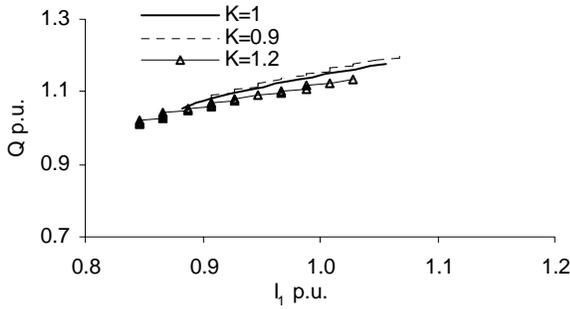
Fig. 15 Variation of reactive power with stator current, terminal voltage =1.2 V<sub>1</sub>, frequency=K f<sub>s</sub>
