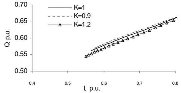
Fig. 13 Variation of reactive power with stator current, terminal voltage =  $V_1$ , frequency= $K f_s$
