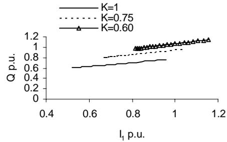
Fig. 12 Variation of reactive power with stator current, terminal voltage =  $1.2 V_1$ , magnetizing reactance= $K X_{mu}$
