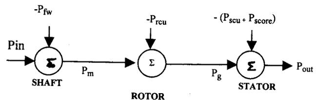
Fig.2 Power flow diagram of induction generator.
