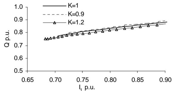
Fig. 14 Variation of reactive power with stator current, terminal voltage =  $1.1 V_1$ , frequency= $K f_s$
