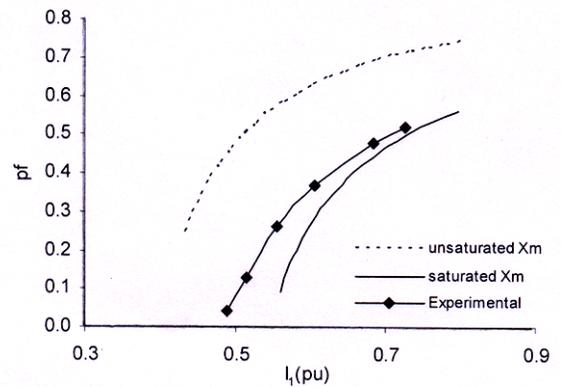
Fig.7 Variation of power factor with stator current
