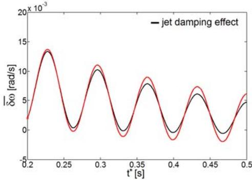
Fig. 9 Induced deviation of the  $\omega$  angular velocity angle vs. time
