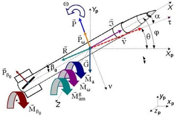
Fig. 1 Longitudinal plane motion of partially guided missile
