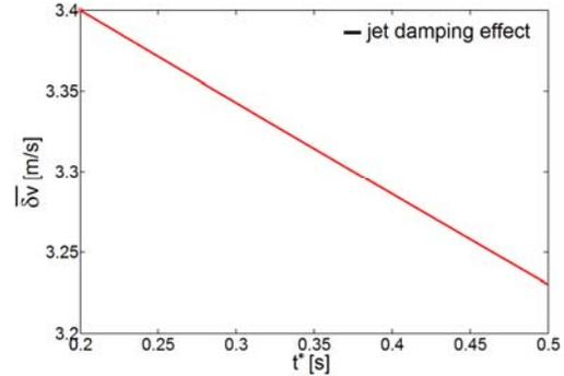
Fig. 5 Induced deviation of the missile speed vs. time
