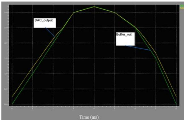
Fig. 5. Analog Buffer circuit tracking performance for large signal input swing
