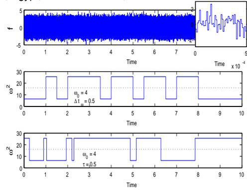
Figure 1: Sample functions of the noises. The top one is a driving force  $f(t)$  where  $\Delta t_f = 0.00001$ . The middle one is a parametric noise of model 1 where  $\Delta t_\omega = 0.5$ . The value can change at integral multiples of  $\Delta t_\omega$ . The bottom one is a parametric noise of model 2 where  $\Delta t_\omega = 0.001$  and  $\tau = 0.5$ .
