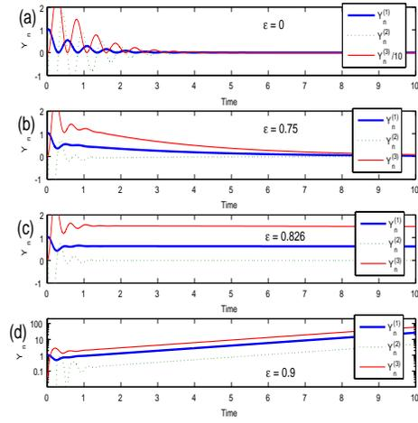
Figure 5: Examples of time evolution of  $\mathbf{Y}_n$ . The parameters are  $\alpha = 1.2$ ,  $\omega_0 = 6$  and  $\tau = 0.2$ . (a) A case for only existing driving force. (b) At  $\epsilon$  near the critical point. (c) At  $\epsilon$  very close to the critical point. (d) At  $\epsilon$  over the critical point. Notice that this is semi-logarithmic graph.
