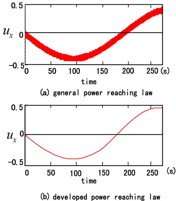
Fig.3 the control input signal
