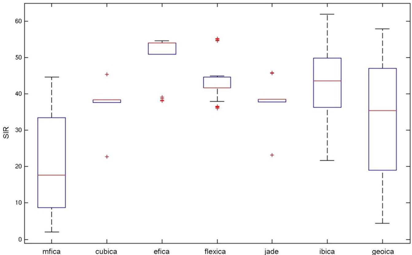
Fig. 3: Mean SIR of 100 runs: Mixture of three speech signals, each with 5000 samples, with linear mixing matrices of size  $3 \times 3$ . In comparison to the standard algorithms, geoica and mfica perform worse, they reach lower SIR values. Efica achieves the best average results.
