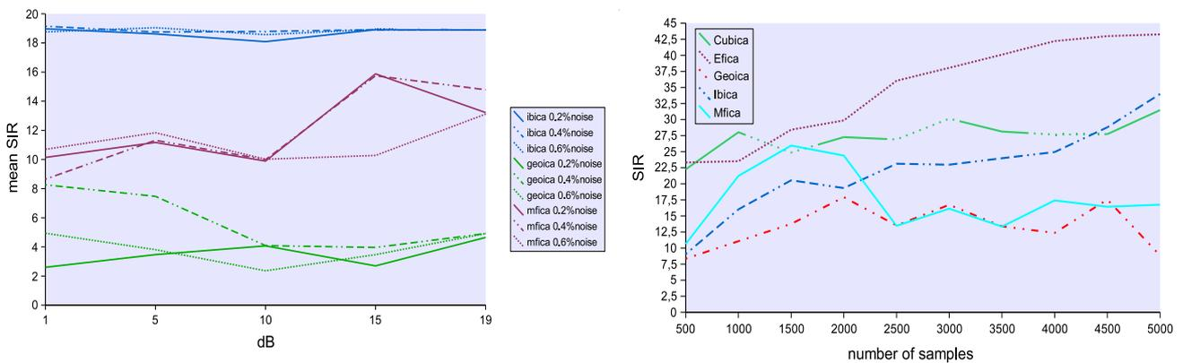
Fig. 2: Each graph: Mean SIR of 100 runs, each with 5000 samples; Left: Mixture of three speech signals, with linear mixing matrices of size  $2 \times 3$ , with different levels of noise. Right: Mixture of four speech signals, with linear mixing matrices of size  $4 \times 4$ , with a decreasing number of samples. For most algorithms the performance lowers with a falling number of samples. Efica outperforms the other algorithms.
