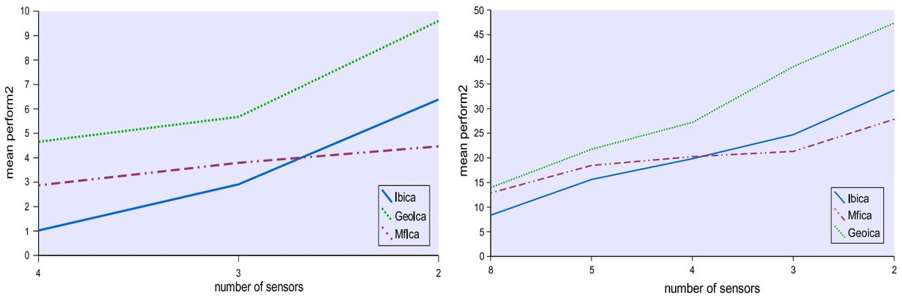
Fig. 1: Mean perform2 of 100 runs: Linear mixture of four (eight) speech signals, each with 5000 samples, with a decreasing number of sensors, from 4 to 2 in the left case and from 8 to 2 in the right case. All three algorithms perform better the more sensors are given. Geoica achieves worse results than ibica and mfica.
