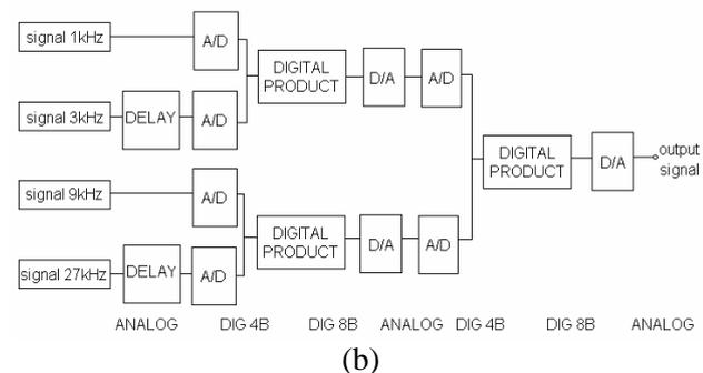
Figure 3 – (a) Optical setup. (b) Block diagram of the electronic system.
