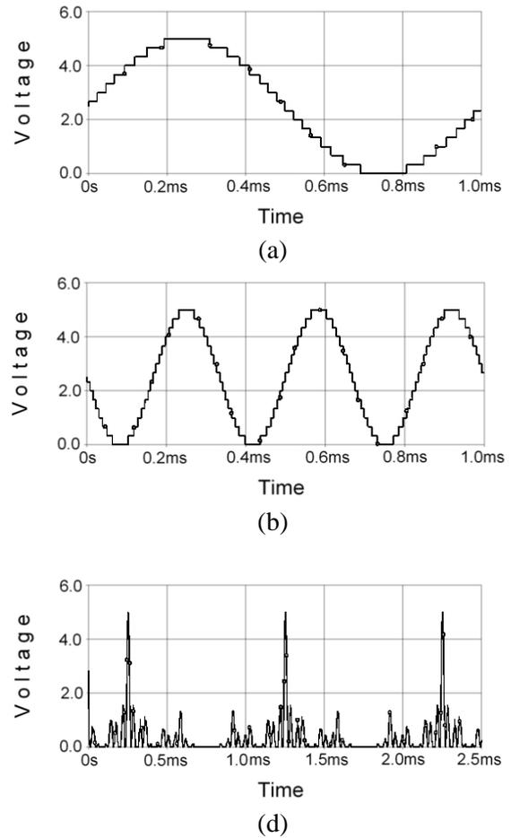
Figure 5 – Voltage vs. Time for the electronic signals for the block diagram of Fig. 3: (a) first periodic component, (b) second periodic component, (c) fractal component with order 3.
