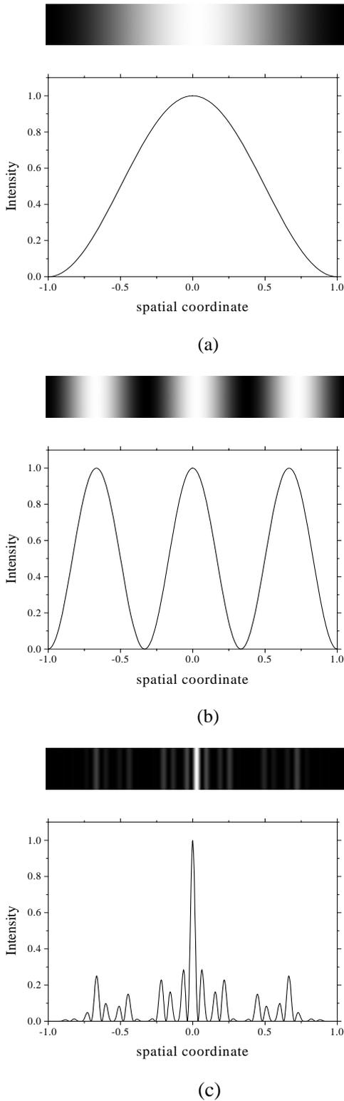
Figure 4 – Intensity vs. spatial coordinate for the interferometers in cascade of Fig. 3: (a) first periodic component, (b) second periodic component, (c) fractal structure with order 3.
