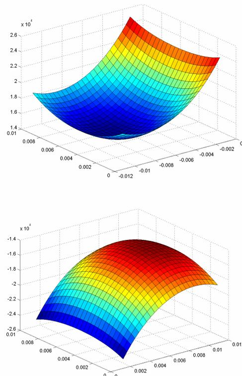
Fig. 1. Distribution of the current density within conductors for  $t=18$  ms
