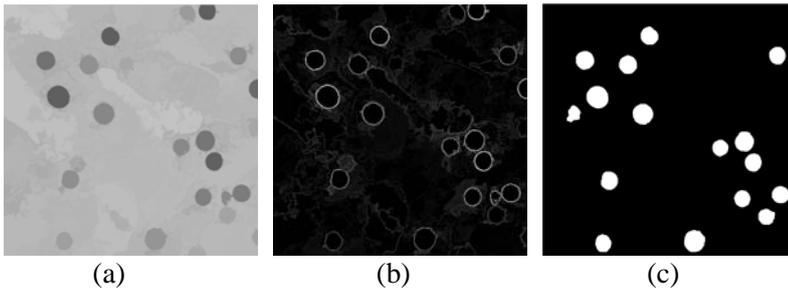
Fig. 3. An example of watershed transform. (a) Result from morphological reconstruction. (b) The gradient image. (c) Result from watershed segmentation.
