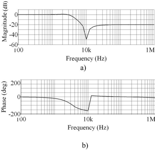
Fig. 5. Amplitude (a) and phase (b) response curves for low-pass rejector filter
