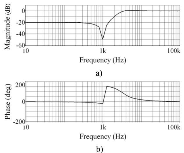
Fig. 4. Amplitude (a) and phase (b) response curves for high-pass rejector filter
