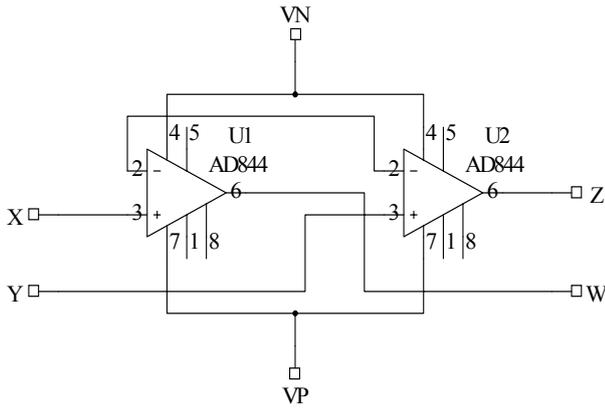
Fig. 2. FTFN built up with two circuits AD 844
