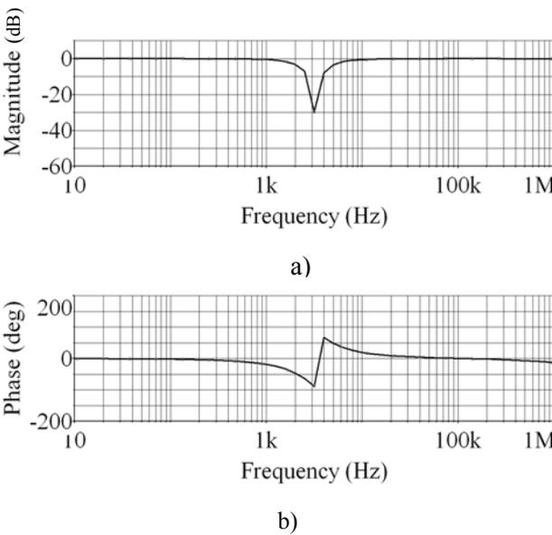
Fig. 6. Amplitude (a) and phase (b) response curves for actual rejector filter
