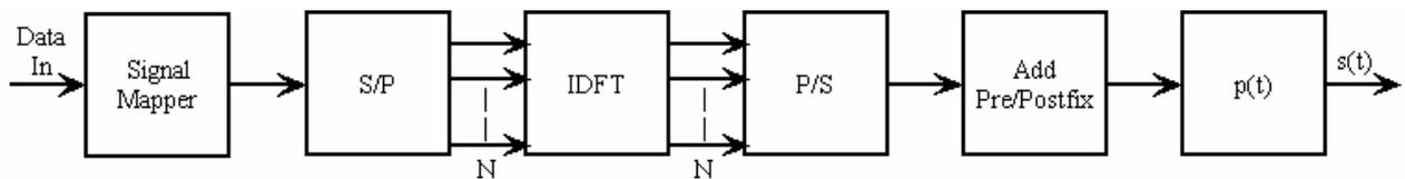
Fig. 1. Block scheme of the transmitter
