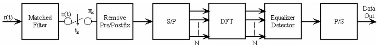
Fig. 2 Block scheme of the receiver
