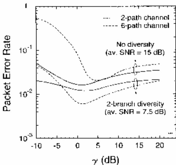
Fig.3. Packet error rate for the proposed communication model
