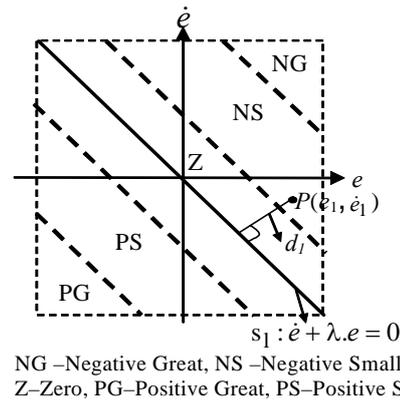
Fig.1. FAM with infinite number of discretization levels
