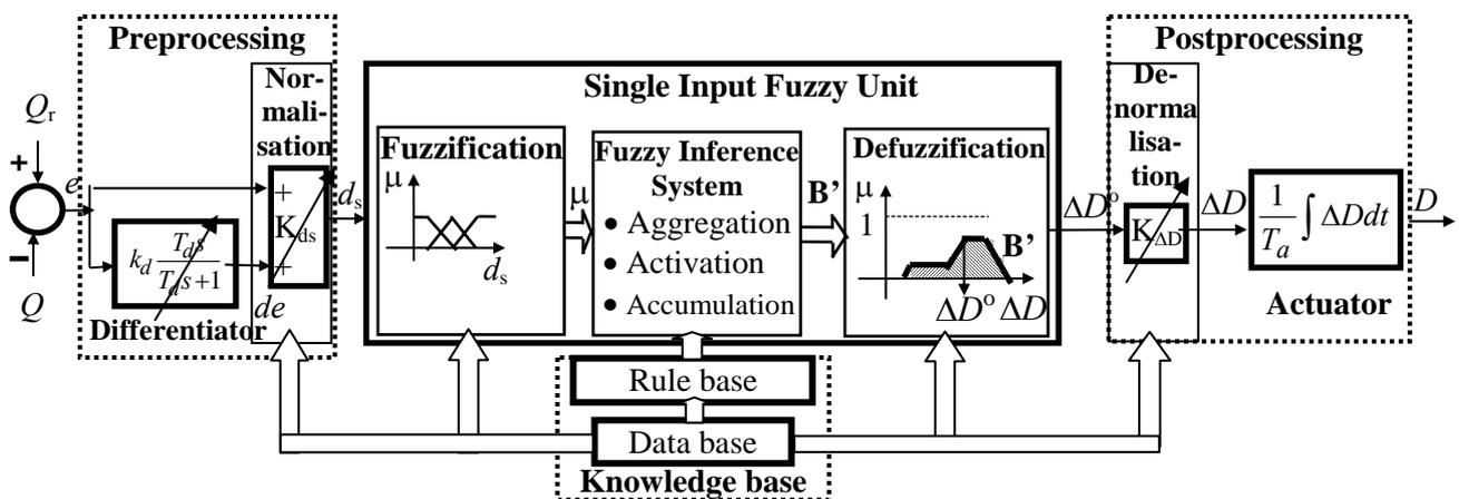
Fig.4. Single input PI fuzzy controller
