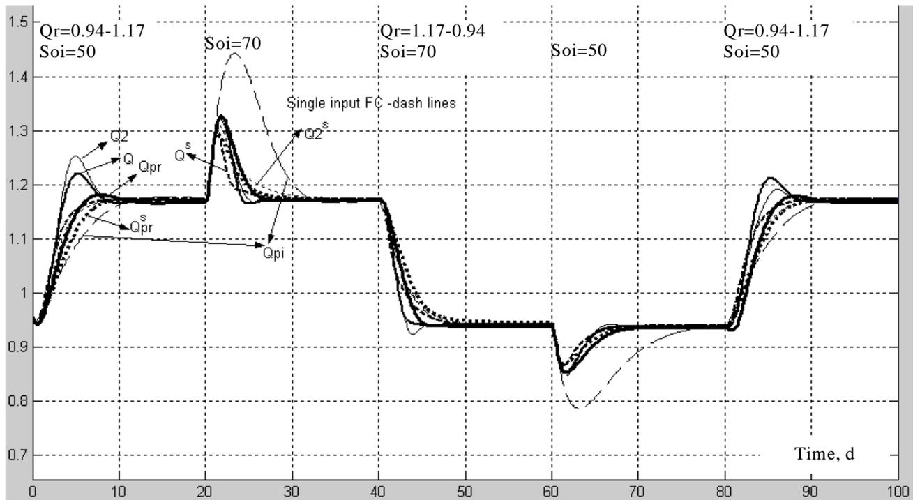
Fig.5. Step responses of closed loop systems with different controllers
