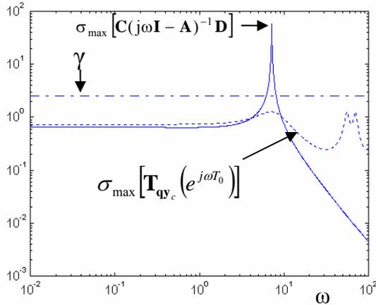
Fig.2. The maximum singular value of  $\mathbf{T}_{qyc}(z)$  over  $\omega$ , for the unsaturated machine and for  $\gamma=2.5$ .
