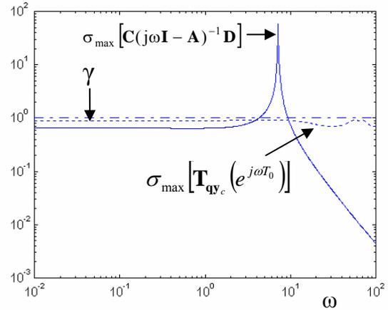
Fig.3. The maximum singular value of  $\mathbf{T}_{qyc}(z)$  over  $\omega$ , for the unsaturated machine and for  $\gamma=1$ .
