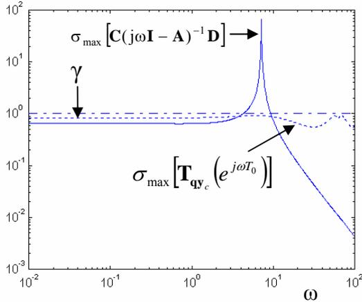
Fig.4. The maximum singular value of  $\mathbf{T}_{qvc}(z)$  over  $\omega$ , for a saturated machine with  $m=1.9$  and for  $\gamma=1$ .
