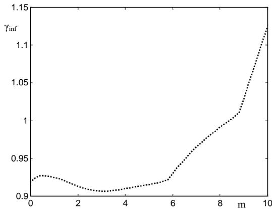
Fig. 5. Minimum achievable disturbance attenuation level  $\gamma_{\text{inf}}$  versus d-axis saturation factor  $m$ .
