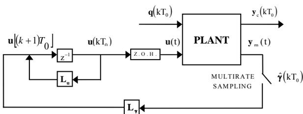
Fig. 1. Control of linear systems using MROCs
