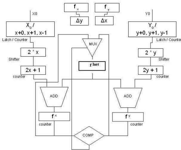
Fig. 4 Block diagram of the hardware implementation of the generator algorithm.
