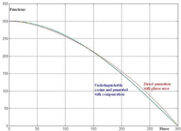
Fig 3. A compensated in time non uniform distribution is not distinguishable from a calculated cosine function simulated in MathLab.
