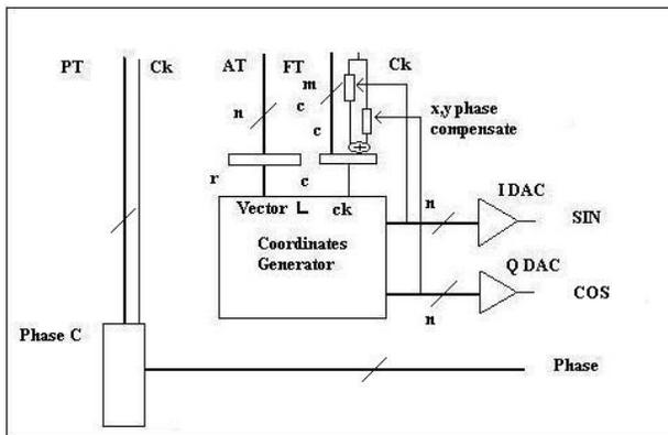
Fig.2 Amplitude based DDS architecture block diagram illustrating the principle.
