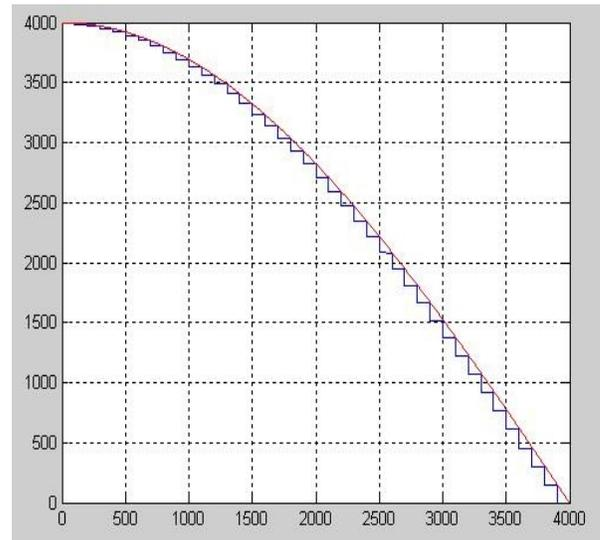
Fig. 5 Simulated delay timing truncated as a trade off between minimal phase error and maximum output frequency.
