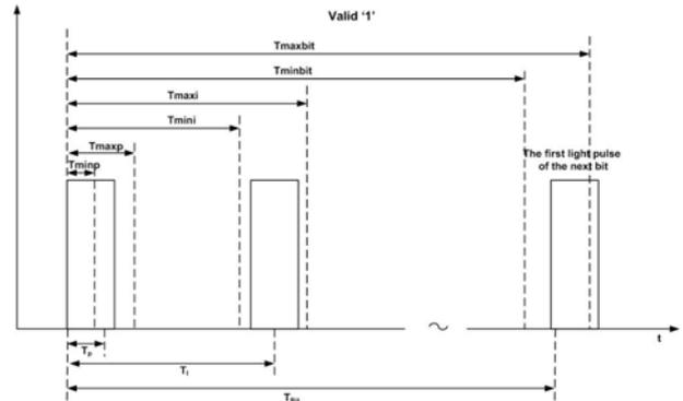
Figure 5: Illustration of the windowing used to avoid the effects of variation of the local frequency.
