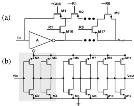
Figure 6: (a) Schematic of the transimpedance amplifier (b) Simplified (power-down transistor is not shown) transistor level schematic of the amplifier of the TIA.
