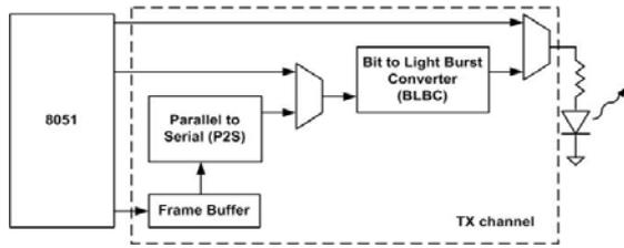
Figure 4: TX channel architecture
