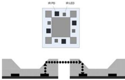
Figure 1: Top and side view of the micromirror and the LED/photodiode structure. The optical link is shown for two robots.
