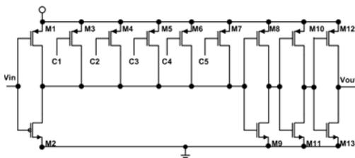
Figure 7: Simplified (power-down transistor is not shown) transistor level schematic of the decision circuit.
