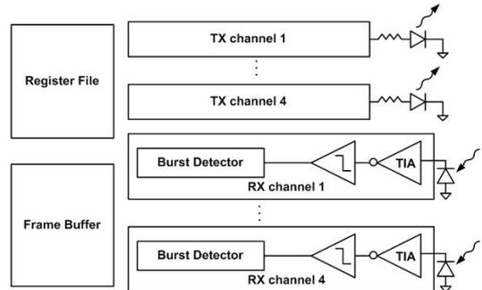
Figure 3: Overall architecture of the transceiver
