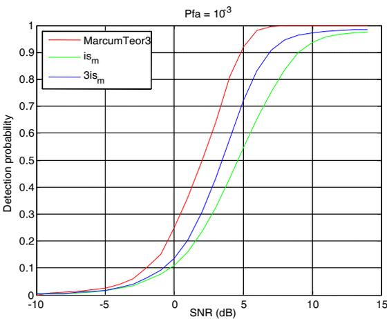
Fig. 9. Detection Probability,  $P_{fa}=10^{-3}$ , Threshold 0.15
