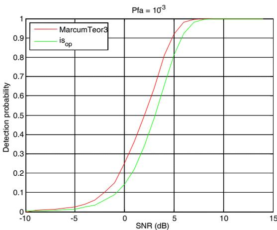
Fig. 13. Detection Probability,  $P_{fa}=10^{-3}$ , Threshold 0.2, The Best Case
