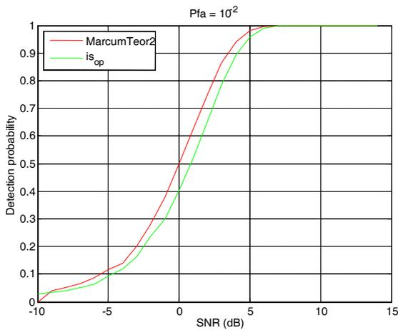
Fig. 12. Detection Probability,  $P_{fa}=10^{-2}$ , Threshold 0.2, The Best Case
