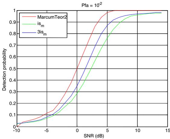
Fig. 4. Detection Probability,  $P_{fa}=10^{-2}$ , Threshold 0.2.
