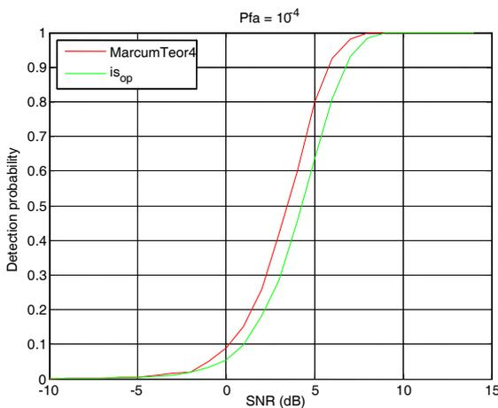
Fig. 14. Detection Probability,  $P_{fa}=10^{-4}$ , Threshold 0.2, The Best Case
