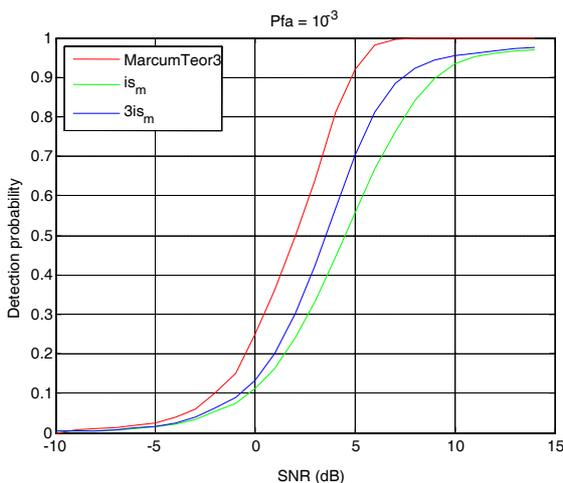
Fig. 5. Detection Probability,  $P_{fa}=10^{-3}$ , Threshold 0.2.
