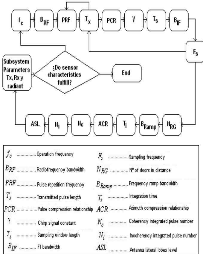
Fig. 2. Calculation Algorithm
