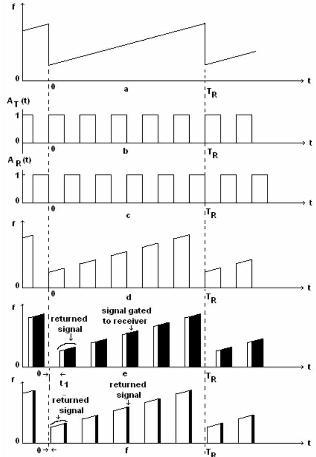
Fig. 1. FMICW technique: (a) Generated FMCW signal, (b) Transmitter gating sequence, (c)gating sequence (complement of transmit sequence), (d) FMICW signal using the gating sequence b, (e) FMICW signal echo from target with two way travel time of  $t_1$  seconds, (f) FMICW signal echo from target with two way travel time of  $t_2$  seconds [5].
