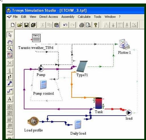
Fig. 3: The TRNSYS Simulation Studio
