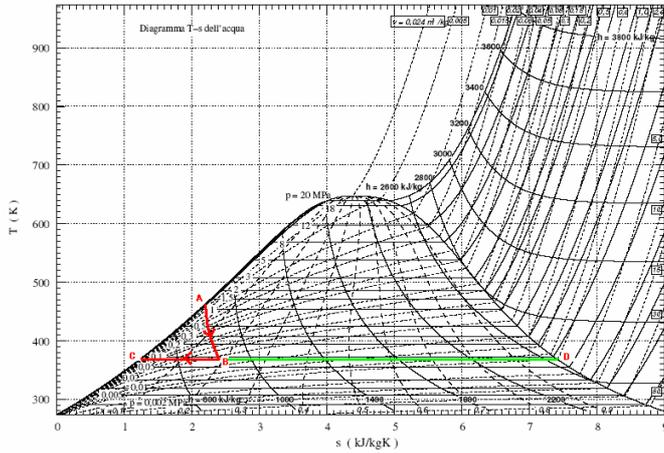
Fig. 2: Water temperature- entropy diagram: transformations of the evaporative chamber.
