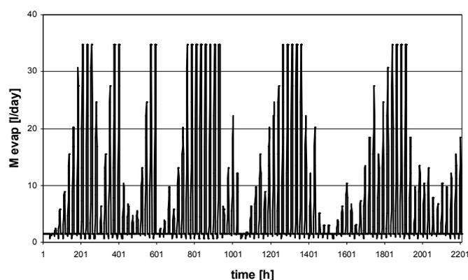
Figure 5: Evaporated mass flow in the spray-type flash evaporator
