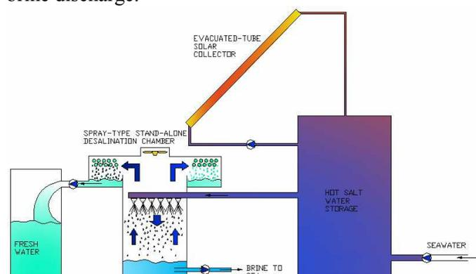
Fig. 1: Schematic of the stand-alone solar desalination plant.
