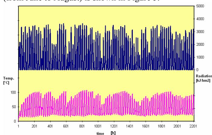
Fig. 4: Solar radiation (upper graph) and solar collector temperatures (lower graph)
