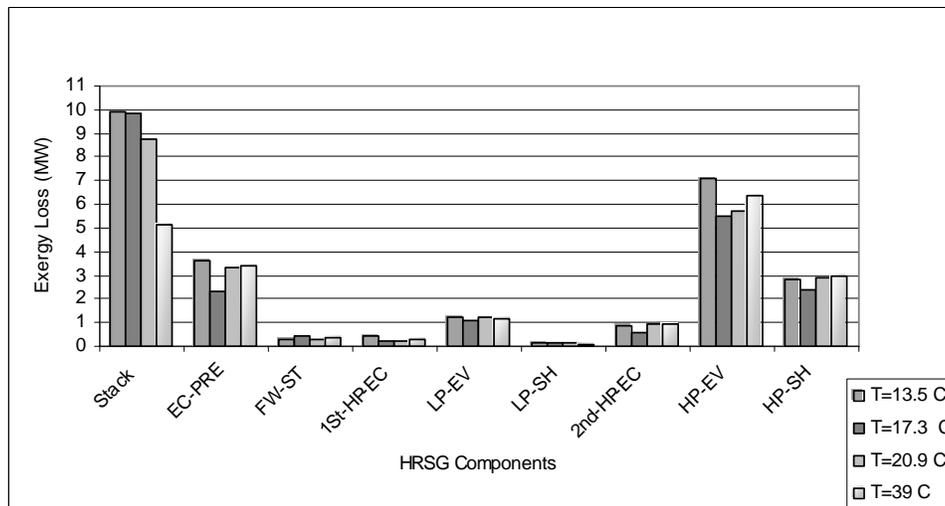
Fig.3 The exergy losses for the HRSG components for the different ambient temperatures for the unfired case
