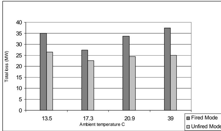
Fig. 2 The comparison of total exergy losses versus ambient temperature for the fired & unfired cases
