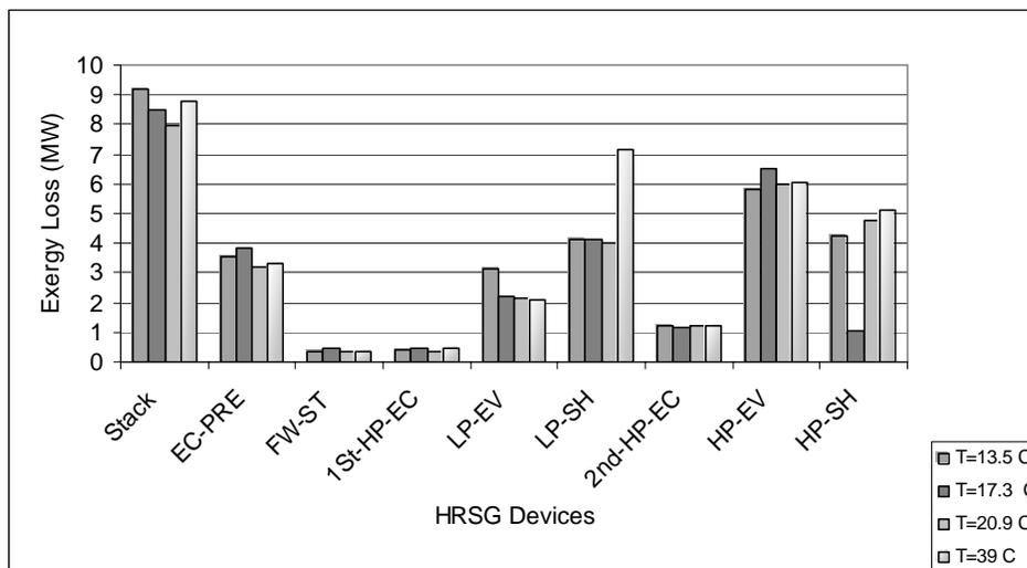
Fig.4 The exergy losses for the HRSG components for the different ambient temperatures for the fired case
