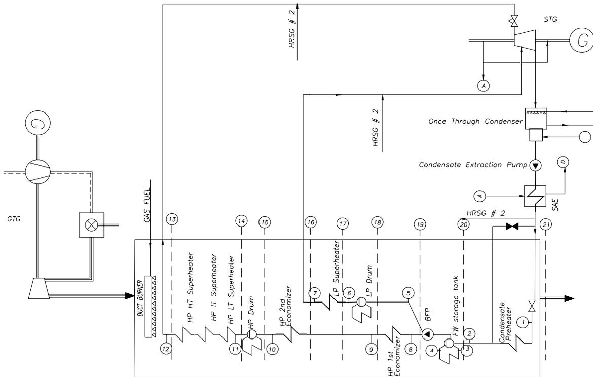
Fig. 1 Schematic of the process flow diagram for the Neka CCPP
