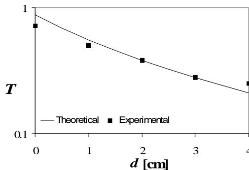
Figure 4: Reactor transmittance as function of suspension thickness, for a catalyst concentration of 0.05 g/L.
