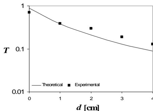
Figure 6: Reactor transmittance as function of suspension thickness, for a catalyst concentration of 0.3 g/L.
