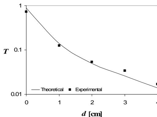
Figure 5: Reactor transmittance as function of suspension thickness, for a catalyst concentration of 0.1 g/L.
