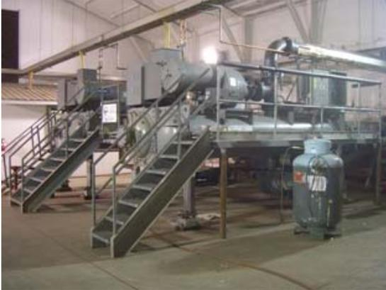
Figure 10. Two ORC power plants (400 kW) at Chena Hot Springs near Fairbanks, AK
