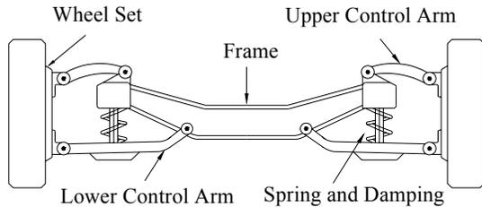
Fig. 1: Schematic of the Suspension Mechanism
