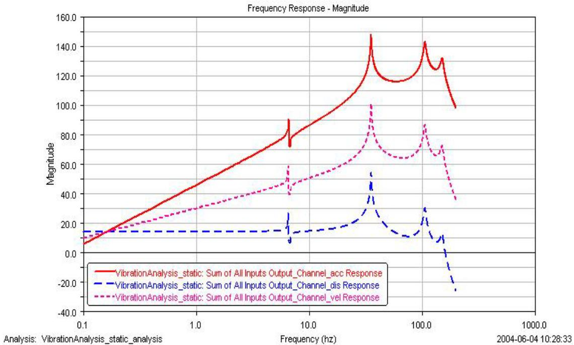
Fig. 3: Frequency Response of the Seat Mass Center
