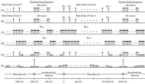
Figure 4: Model of Multi-Rate Quasi-Synchronous CDMA System.
