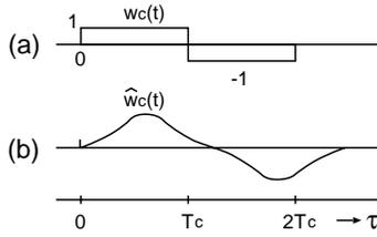
Figure 2: Chip waveforms.
