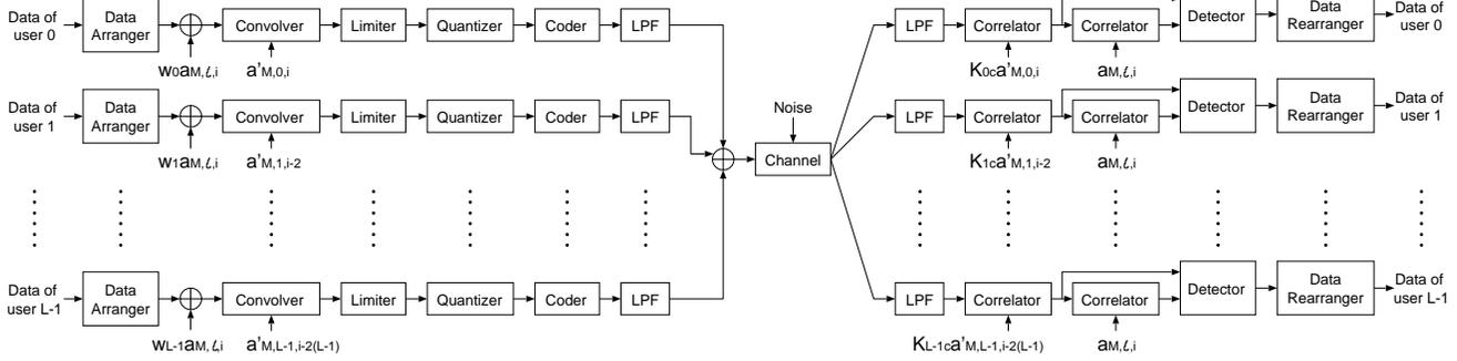
Figure 3: Model of Multi-Rate Quasi-Synchronous CDMA System.
