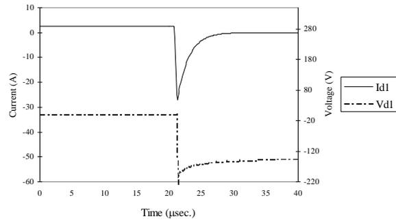
Figure 4: Simulation result: Diode current and voltage waveforms
