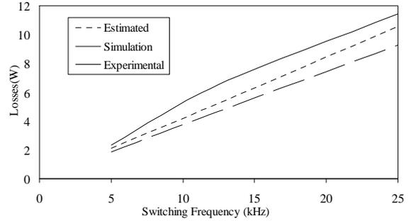
Figure 7: Diode power losses
