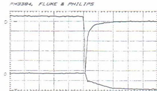
Figure 5: Experimental result: diode current and voltage waveforms during diode turn-off transient (5 A/div 100 V/div & 5 µsec/div)
