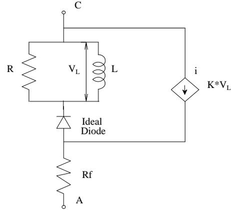
Figure 2: Proposed Model for the diode reverse recovery
