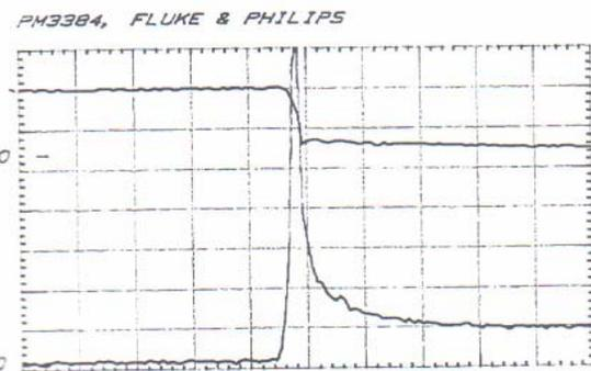
Figure 6: Experimental result: IGBT current and voltage waveforms during switch turn-on transient (2.5 A/div 100 V/div & 2.5 µsec/div)
