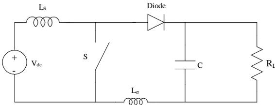
Figure 3: DC boost converter
