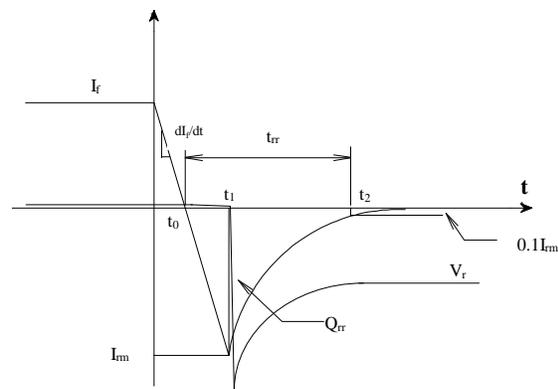
Figure 1: Diode reverse recovery current and voltage waveforms
