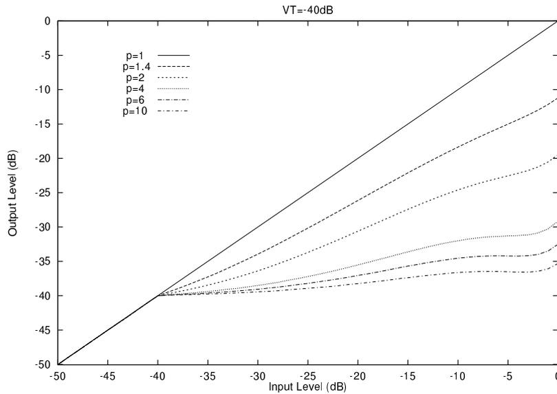
Figure 7: The compression characteristics by VHDL simulation.
