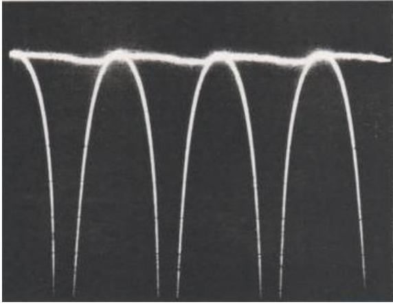
Figure 6: The gain smoothed by attack/release circuit.
