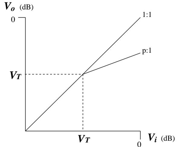
Figure 2: Compression characteristic.
