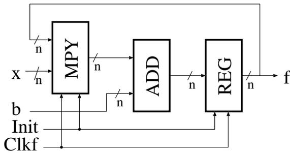
Figure 4: Arithmetic circuit for computing a polynomial expression.
