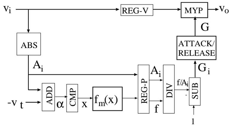
Figure 3: Architecture of the proposed compressor.
