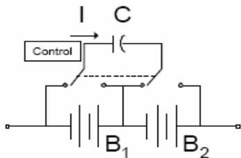
Figure 7, Charge Shuttling Between Two Cells
