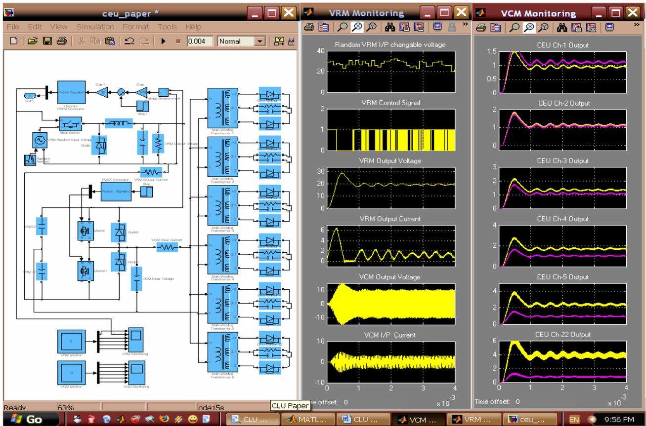
Figure 16, the CEU Simulink model and testing results with a resistive loading
