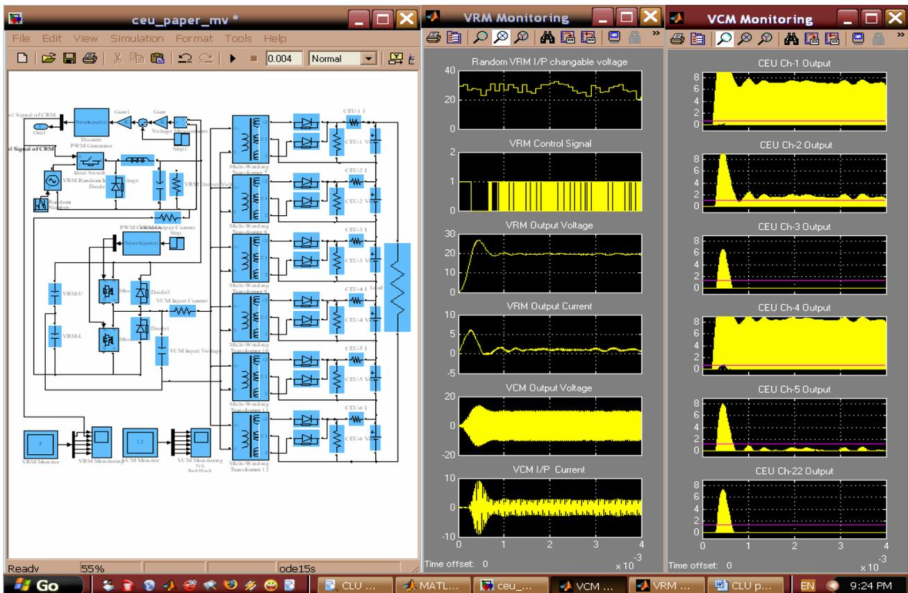
Figure 17, the CEU Simulink model and testing results with a battery cell loading
