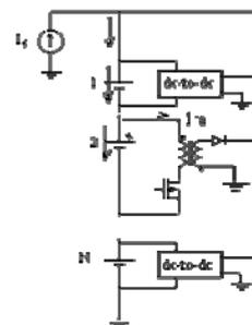
Figure 10, Charge equalization using isolated flyback dc-to-dc converter
