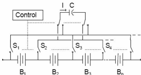
Figure 6, Flying Capacitor Charge Shuttling
