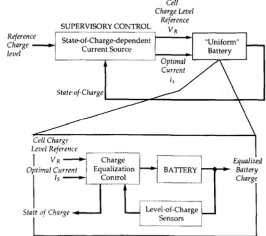
Figure 2, topology of charge equalization by two-level control mechanism
