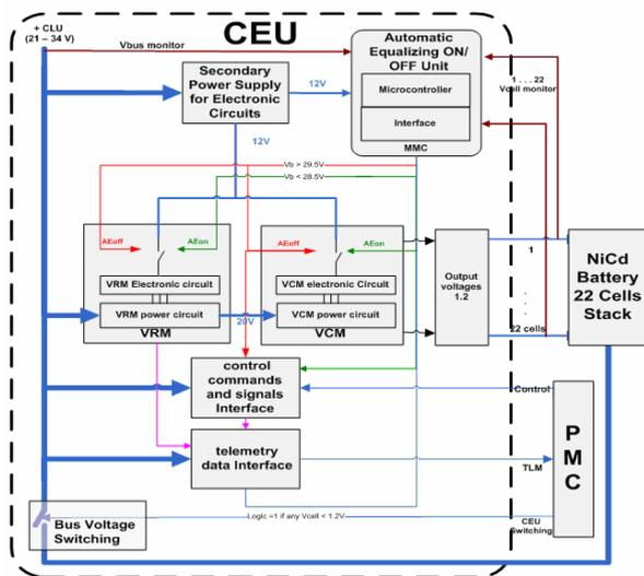
Figure 15, CEU functional block diagram
