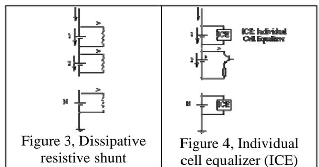
Figure 3, Dissipative resistive shunt
