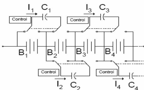
Figure 8, Charge Shuttling with Several Cells
