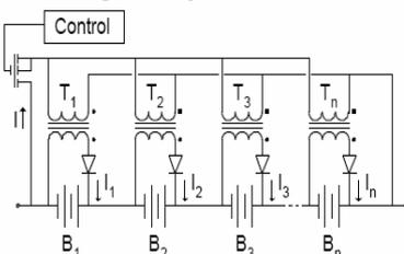
Figure 13, Multiple Transformer
