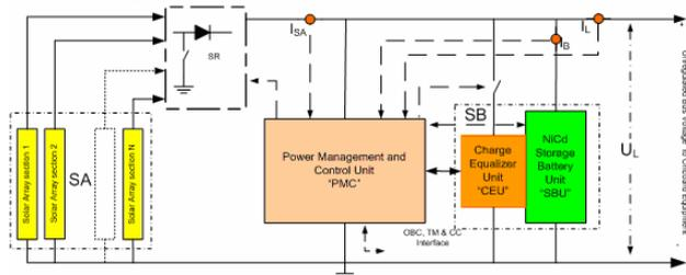
Figure 1, Block diagram of the proposed Microsatellite EPS (OBC stands for On-Board Computer, TM stands for Telemetry, and CC stands for Control Commands)
