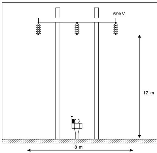
Fig.7 Test domain for mobile-phone-human interfacing with an overhead HV power transmission line
