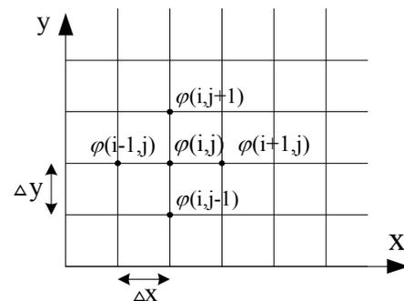
Fig.3 Discretization of 2D domain
