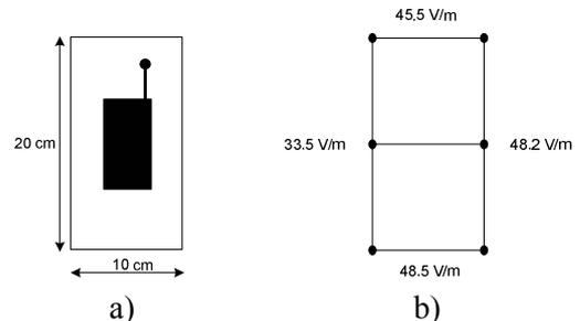
Fig.5 Mobile phone discretization for FDM
