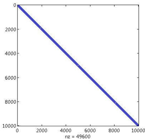
Fig.13 Sparsity of the system coefficient matrix
