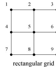
Fig.2 Domain discretization of the FDM
