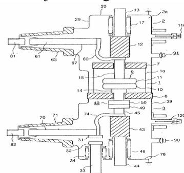
Fig.1 the structure of VIS (without bus) [1]
