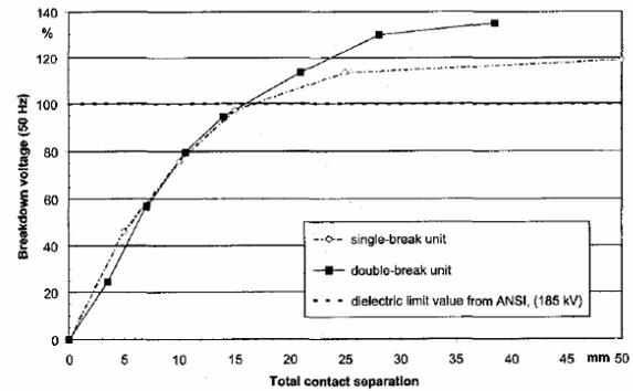
Fig.4 AC voltage limit of double and single-break units as a function of contact separation [5]
