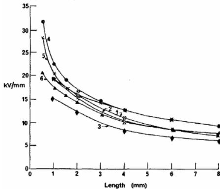
Fig.6 Relationship between the flashover field strength and insulator's length [11]
