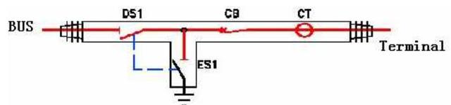
Fig.8 typical structure of switchgear (CB: circuit breaker, DS: disconnector switch)
