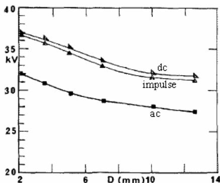
Fig.7 Relationship between flashover voltage and insulator's diameter [11]
