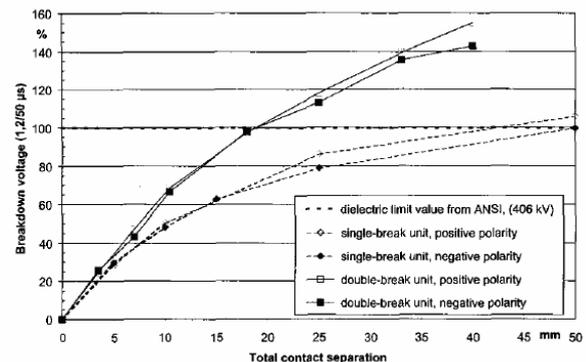
Fig.5 Lightning impulse voltage limit for double and single-break units as a function of contact separation[5]
