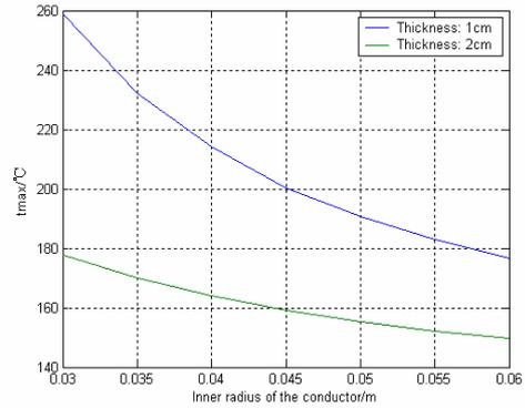
Fig.10 Relationship between tmax and radius of the conductor
