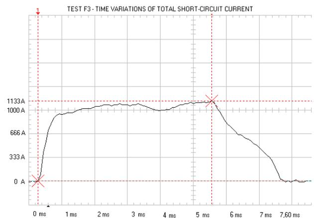
fig. 7 – time variations of short-circuit current in location F3
