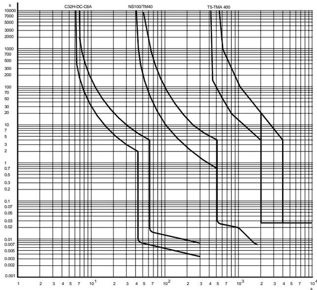
Fig. 4 – Breaking I-t curves for circuit breakers situated in three protection level
