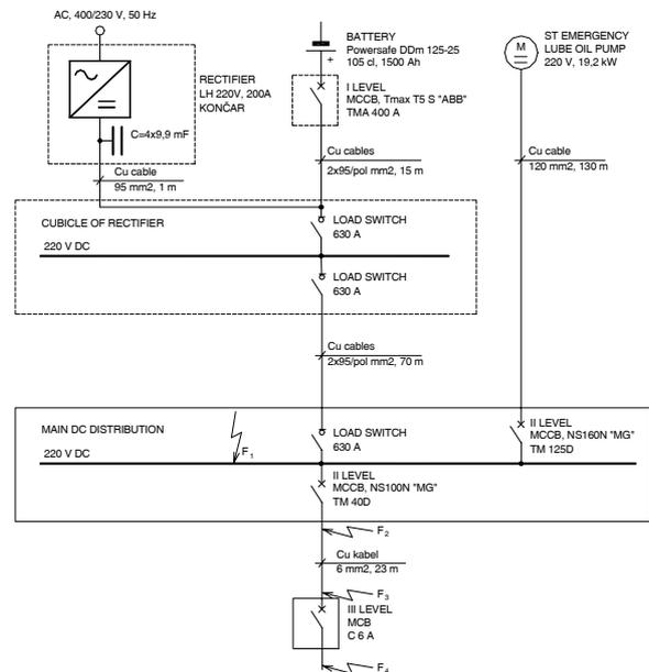
Fig. 2 – block diagram of the 220 VDC auxiliary system in TPP Rijeka
