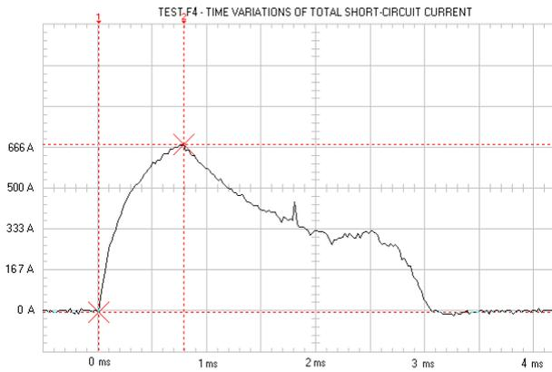
fig. 8 – time variations of short-circuit current in location F4
