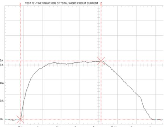
fig. 6 – time variations of short-circuit current in location F2
