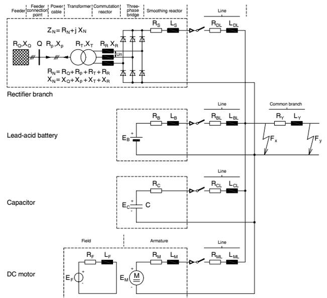
Fig. 1 – equivalent circuit diagram of the DC auxiliary system
