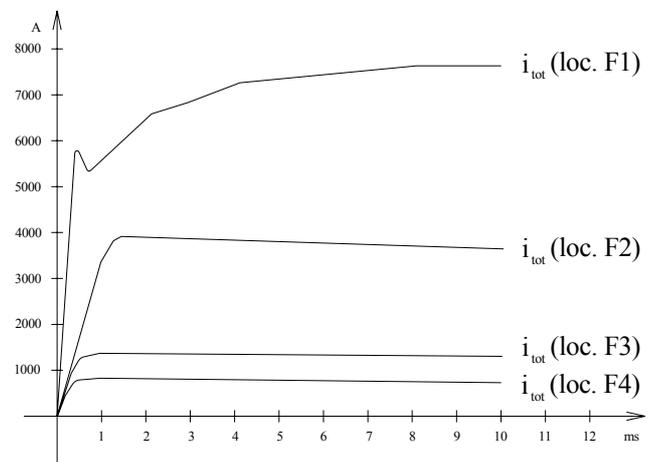
Fig. 3 – Time variation of total short-circuit current in locations F1-F4 during first 10 ms
