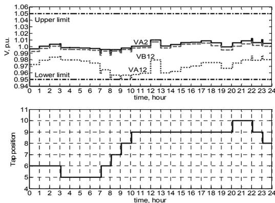
Fig. 6 Voltage profiles for Buses A2, A12 and B12, and tap positions of ULTC by Lookup-table method (DG of 0.9MW, P.F.=0.95 leading @ Bus A12)
