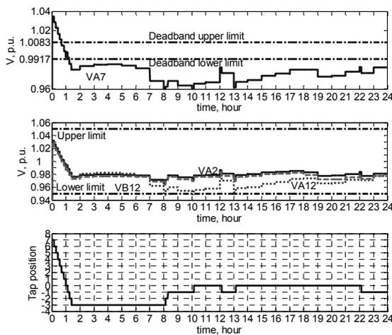
Fig. 9 Voltage profiles of Buses A2, A12, B12 and CVP(A7), and tap positions of ULTC by LDC (DG of 6MW, P.F.=0.85 lagging @ Bus A3)
