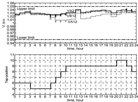
Fig. 5 Voltage profiles for Buses A2, A12 and B12, and tap positions of ULTC by Lookup-table method (DG of 6MW, P.F.=0.85 lagging @ Bus A3 )
