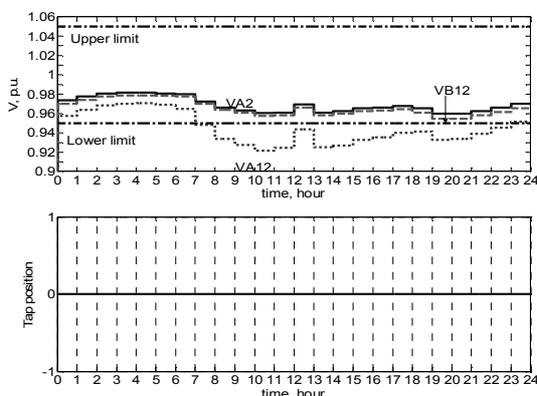
Fig. 4 Voltage profiles of Buses A2, A12 and B12, and tap position of ULTC (without voltage regulation)
