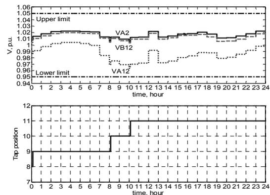
Fig. 8 Voltage profiles for Buses A2, A12 and B12, and tap positions of ULTC by Voltage-based method (DG of 0.9MW, P.F.=0.95 leading @ Bus A12)
