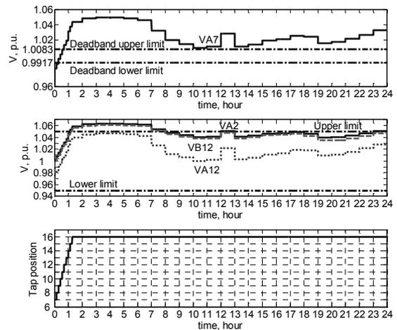
Fig. 10 Voltage profiles of Buses A2, A12, B12 and CVP(A7), and tap positions of ULTC by LDC (DG of 0.9MW, P.F.=0.95 leading @ Bus A12)
