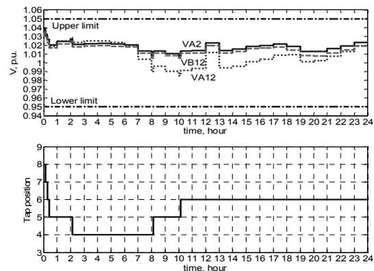
Fig. 7 Voltage profiles for Buses A2, A12 and B12, and tap positions of ULTC by Voltage-based method (DG of 6MW, P.F.=0.85 lagging @ Bus A3 )
