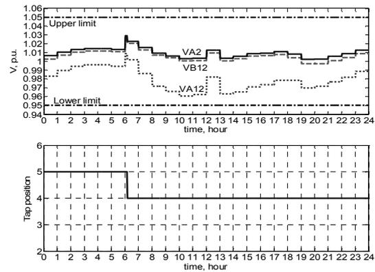
Fig. 12 Voltage profiles of Buses A2, A12 and B12, and tap positions of ULTC by Taipower's RPDC method (DG of 0.9MW, P.F.=0.95 leading @ Bus A12)
