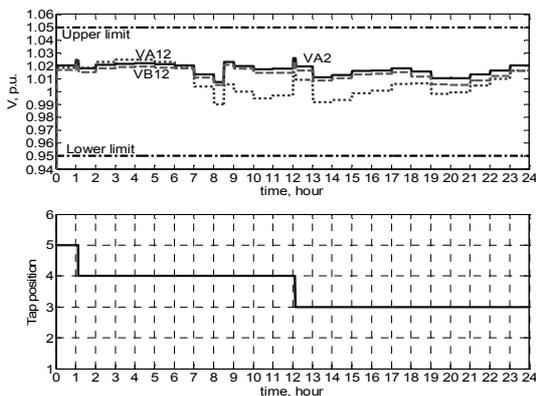
Fig. 11 Voltage profiles of Buses A2, A12 and B12, and tap positions of ULTC by Taipower's RPDC method (DG of 6MW, P.F.=0.85 lagging @ Bus A3)
