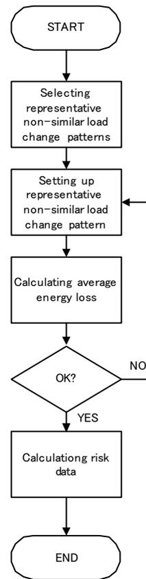
**Fig. 3.** Flowchart for calculating risk data in non-similar load change patterns.
