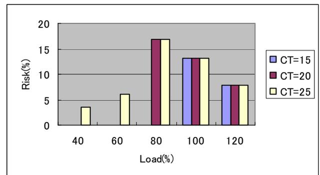
Fig. 6. Change of discrete risk functions by CT(fault clearing time).
