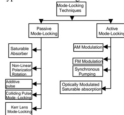
Fig.1: Types of mode locking
