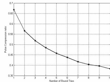
Fig. 5: Pulse compression ratio corresponding to number of round trips
