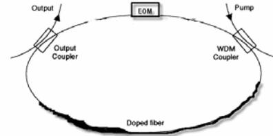
Fig.3: Block diagram of an actively modelocked fiber ring laser
