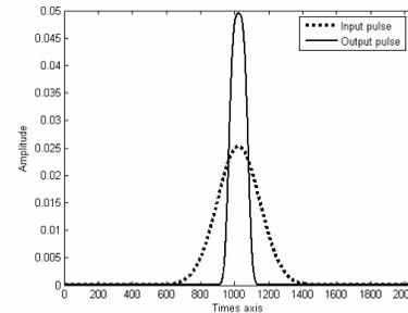
Fig. 4: seed pulse and Mode-locked output pulse
