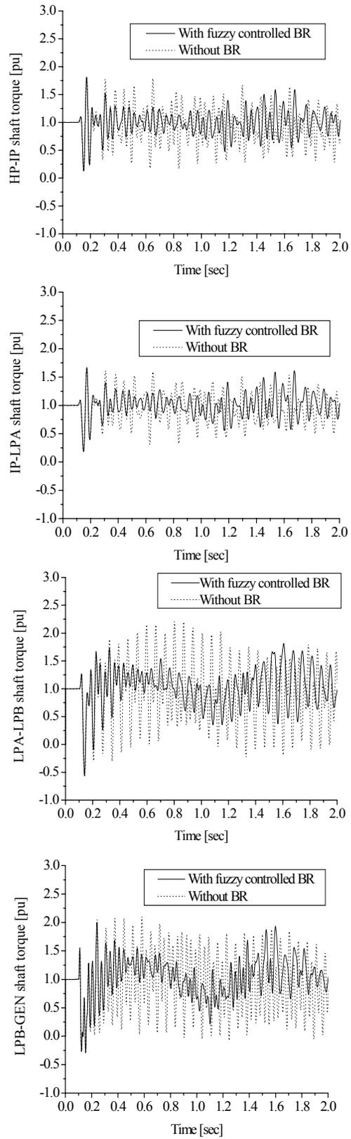
Fig. 7. Shaft torsional torque responses of generator G1 for 3LG fault at point A considering a communication delay of 20 msec.
