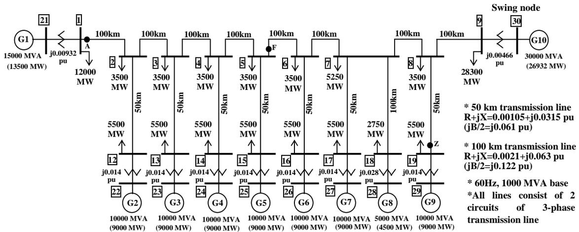
Fig. 1. IEEJ WEST 10-machine model system.
