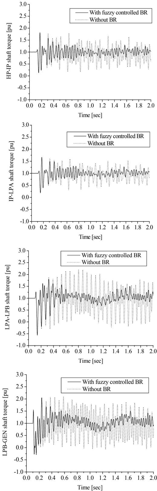
Fig. 6. Shaft torsional torque responses of generator G1 for 3LG fault at point A without considering communication delay.
