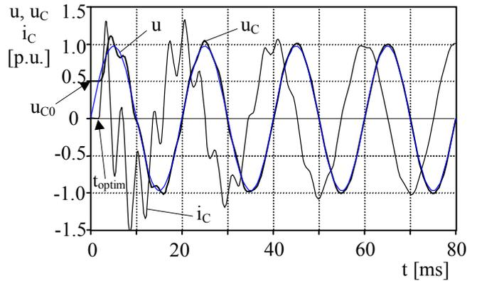
**Fig. 7** The voltage  $u_c$  and current  $i_c$  evolution at the capacitor connection, for  $u_{c0}=0.5U_{Cm}$
