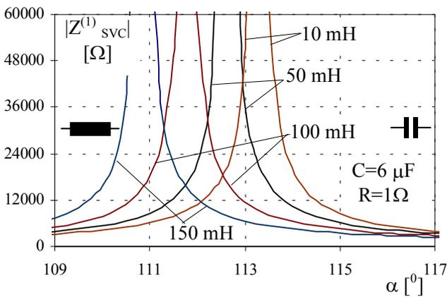
**Fig. 5** SVC fundamental impedance for different values of inductance  $L_c$
