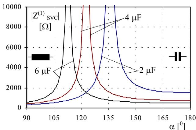
Fig. 2 SVC fundamental impedance for various values of the  $C$
