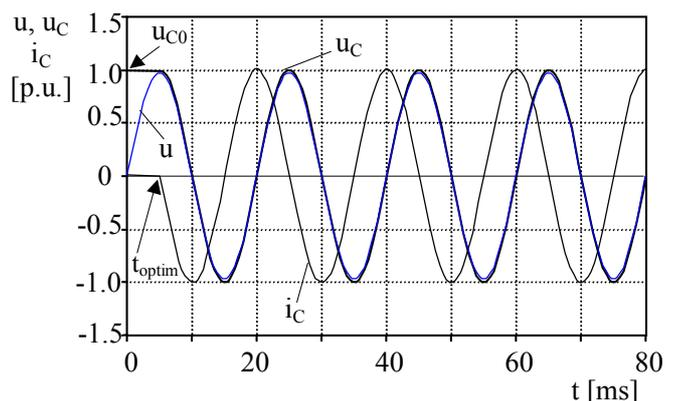
**Fig. 8** The voltage  $u_c$  and current  $i_c$  evolution at the capacitor connection, for  $u_{c0}=U_{Cm}$
