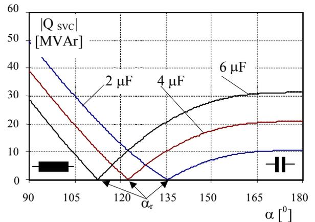
Fig. 3 SVC reactive power for different values of the  $C$  capacitor
