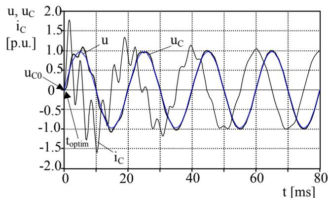
**Fig. 6** The voltage  $u_c$  and current  $i_c$  evolution at the capacitor connection, for  $u_{c0}=0$
