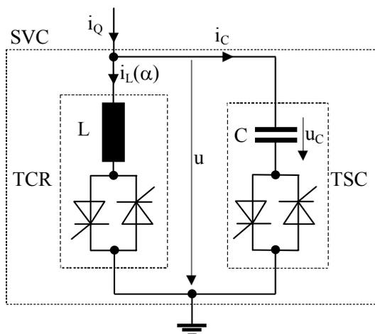
Fig. 1 Shunt compensator scheme – SVC
