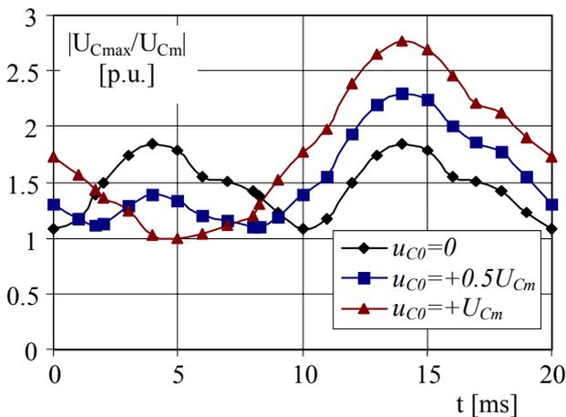
**Fig. 10** Maximum overvoltages on capacitor in function of the charging voltage and the connection moment
