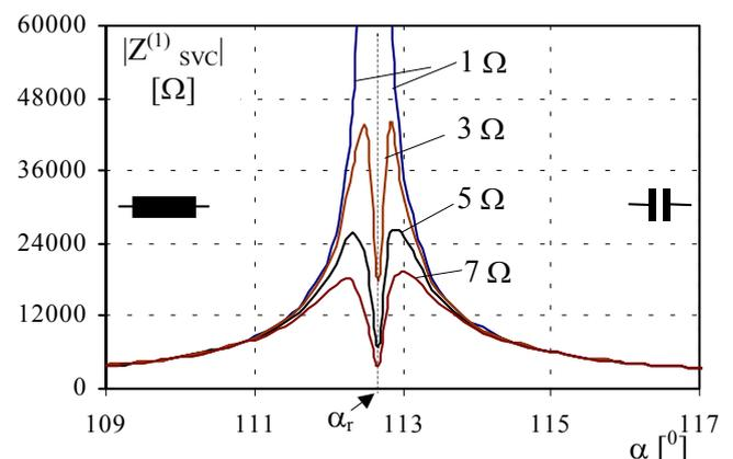
Fig. 4 SVC fundamental impedance for various values of the  $R$
