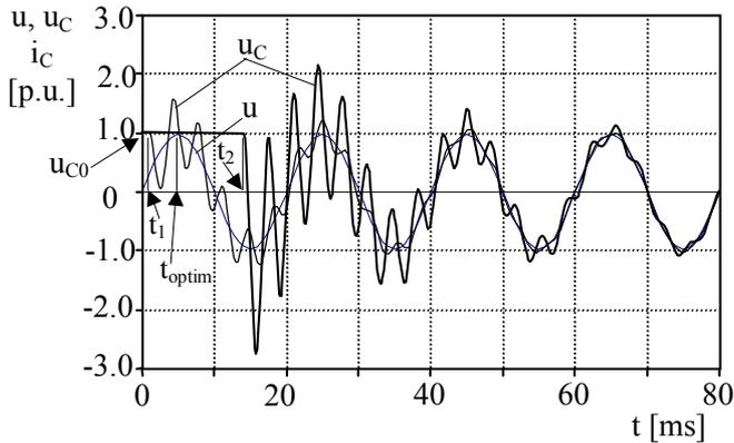
**Fig. 9** The  $u_c$  voltage evolution on the capacitor at  $u_{c0}=U_{Cm}$  and two different connection moments
