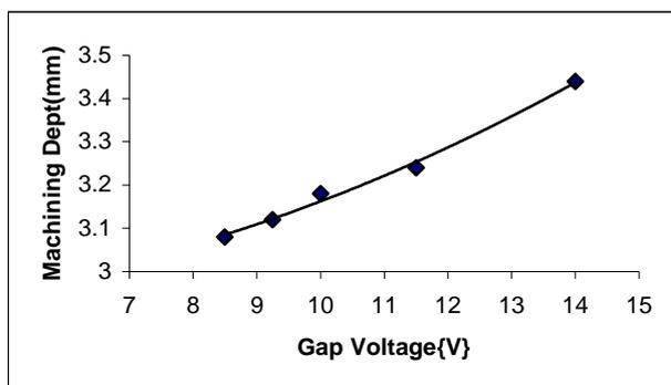
Fig.6: Variations of machining dept with gap voltage
