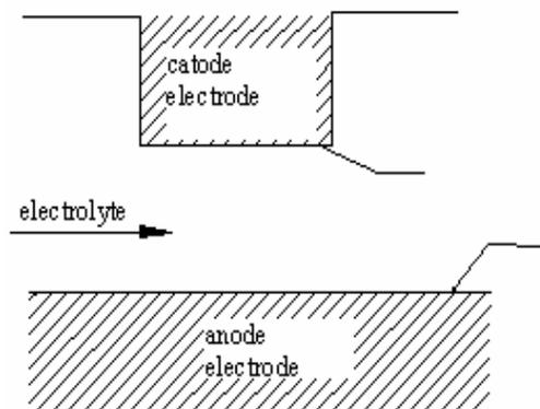
Fig. 1: Machining gap and its boundary condition
