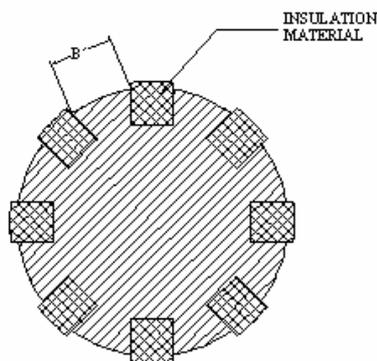
B: Machining width on the surface of tool
