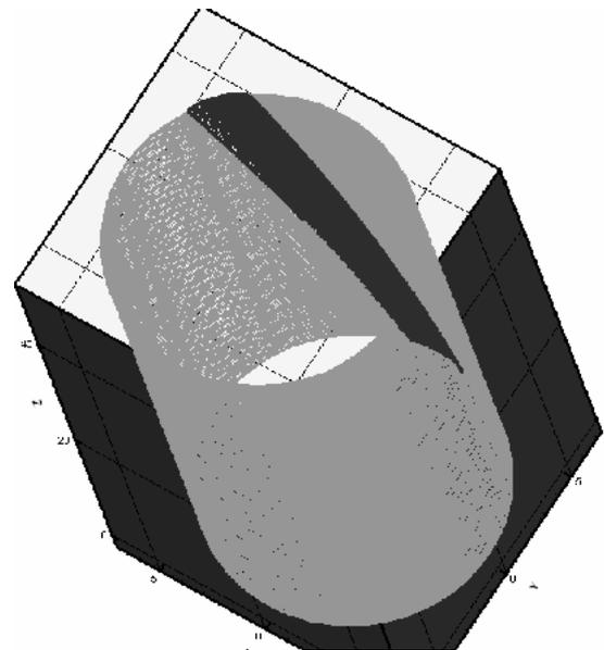
Fig.5: Schematic of simulated helically gun pipe's rifle slot
