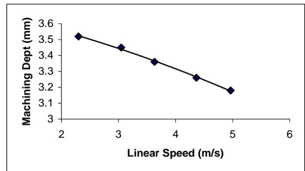
Fig.7: Variations of machining dept with tool's linear speed
