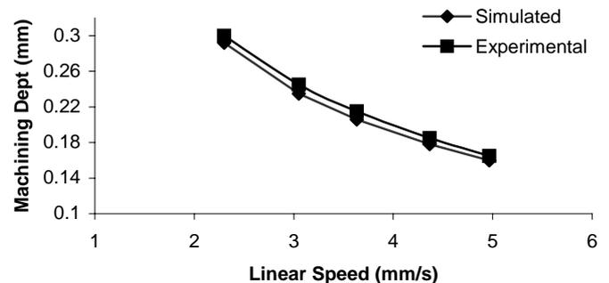
Fig. 8: Simulated and experimental results of machining dept variations with tool's speed
