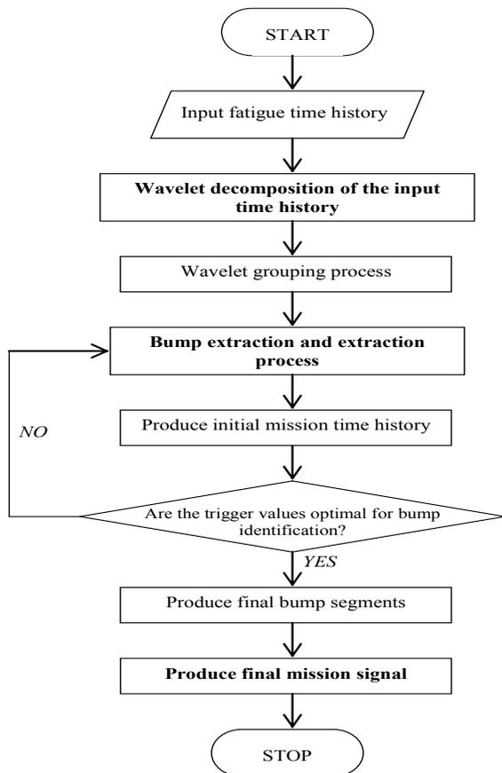
Fig. 1. Flowchart of the WBE algorithm
