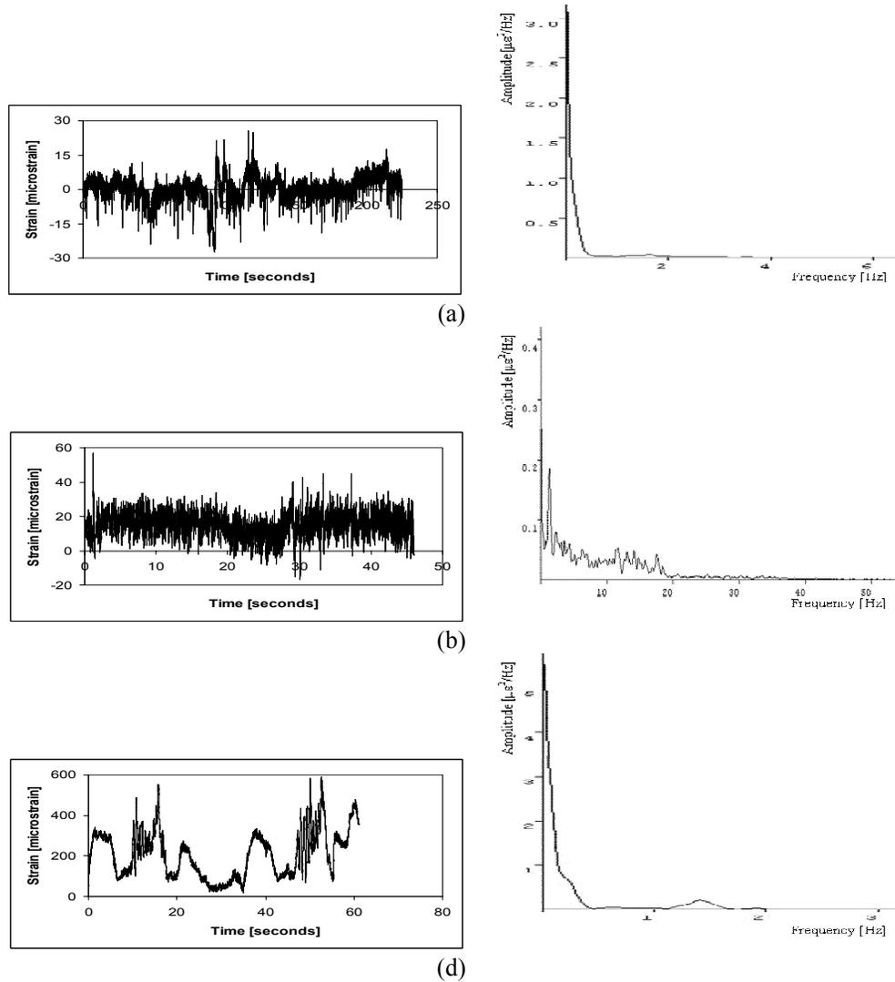
Fig. 3. Time histories and power spectral densities of the original fatigue road loadings: (a) T1, (b) T2, (c) T3.
