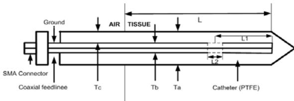
Fig.1 Basic schematic of the general applicator
