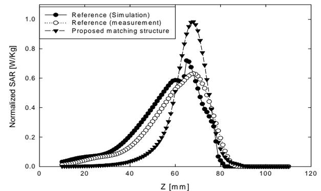
Fig.4 SAR comparison between the general applicator and the proposed matching applicator at 2.45GHz
