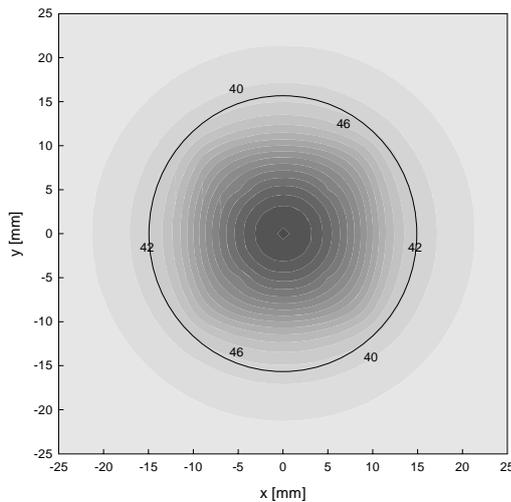
Fig.8 Temperature contour plot on the xy-plane passing through the first slot of the array applicator
