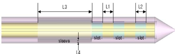
Fig.5 Schematic of 3-slot sleeve antenna
