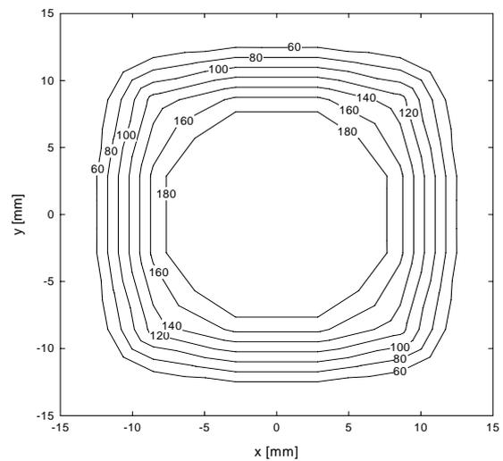
Fig.7 SAR contour plot on the xy-plane passing through the 4-applicator for 1 Watt of radiated power with 10 mm applicator spacing
