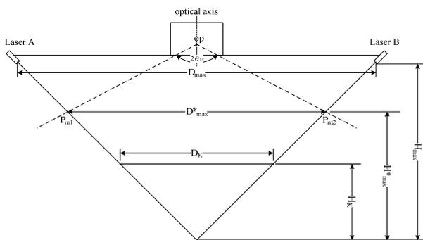
Fig. 1 Schematic diagram illustrating the triangular measuring method.
